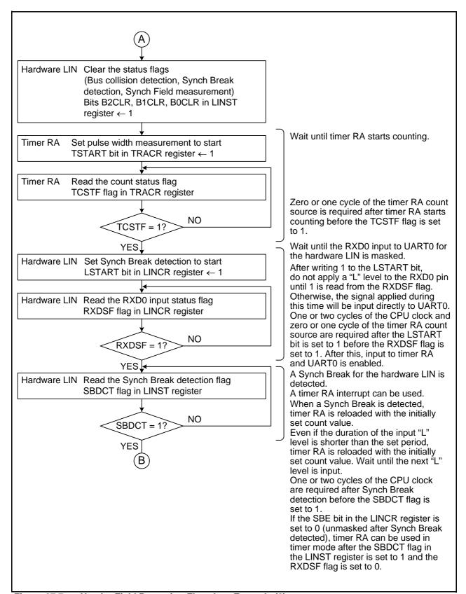
Figure 27.7 Header Field Reception Flowchart Example (2)
