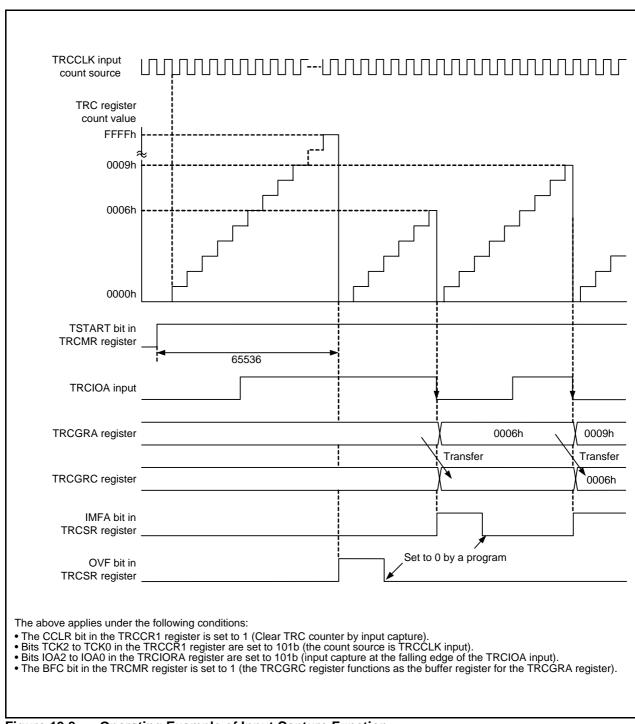
Figure 19.8 Operating Example of Input Capture Function
