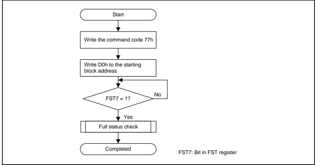
Figure 31.14 Lock Bit Program Flowchart
