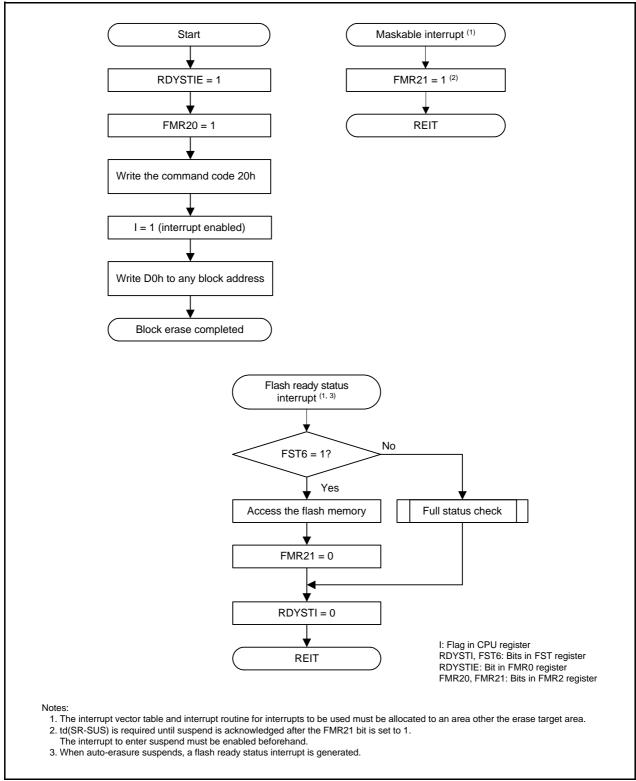
Figure 31.13 Block Erase Flowchart (Flash Ready Status Interrupt Enabled and Suspend Enabled)
