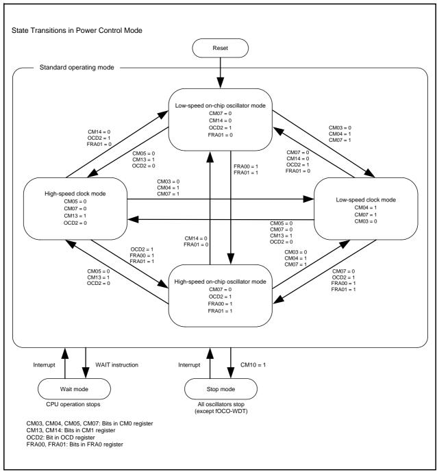
Figure 9.9 State Transitions in Power Control Mode
