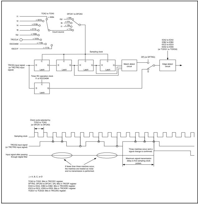
Figure 19.5 Digital Filter Block Diagram
