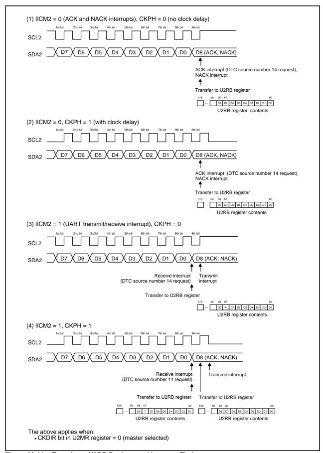
Figure 23.14 Transfer to U2RB Register and Interrupt Timing
