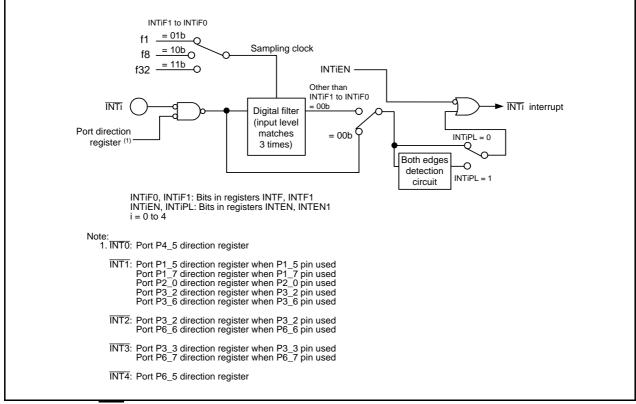
Figure 11.9 INTi Input Filter Configuration
