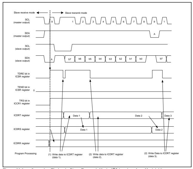
Figure 26.9 Operating Timing in Slave Transmit Mode (I<sup>2</sup>C bus Interface Mode) (1)
