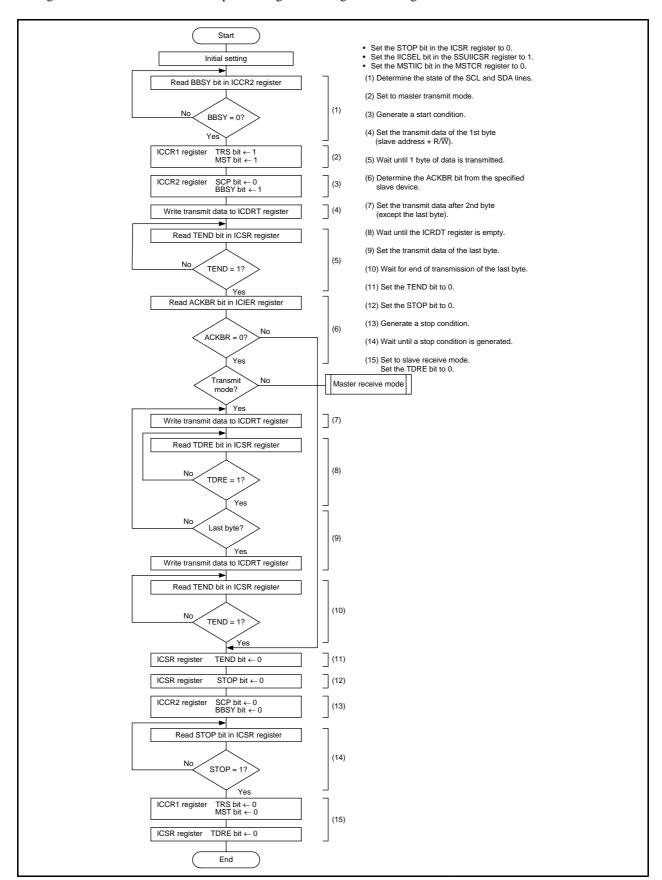
Figure 26.16 Register Setting Example in Master Transmit Mode (I<sup>2</sup>C bus Interface Mode)
