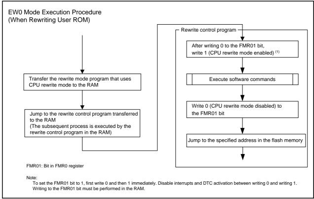
Figure 31.5 How to Set and Exit EW0 Mode
