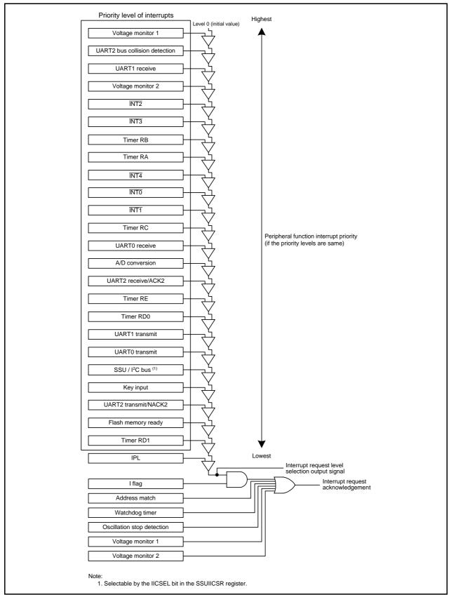
Figure 11.8 Interrupt Priority Level Selection Circuit
