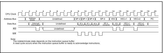
Figure 11.3 Time Required for Executing Interrupt Sequence
