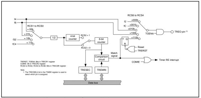
Figure 21.4 Block Diagram of Output Compare Mode
