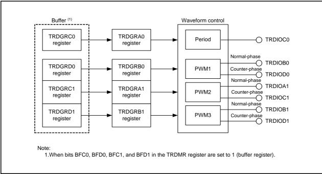
Figure 20.17 Block Diagram of Reset Synchronous PWM Mode
