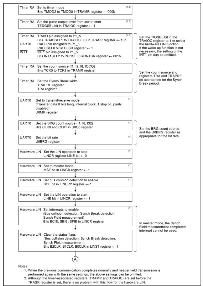
Figure 27.3 Header Field Transmission Flowchart Example (1)
