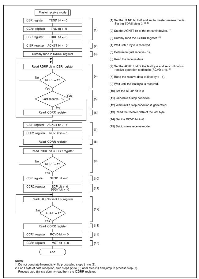
Figure 26.17 Register Setting Example in Master Receive Mode (I<sup>2</sup>C bus Interface Mode)
