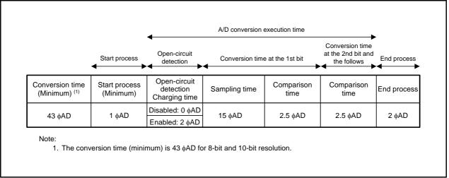
Figure 28.3 A/D Conversion Cycles ( $\phi$ AD = fAD)
