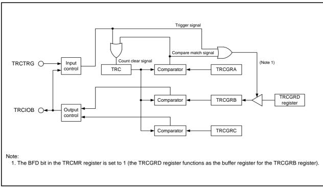
Figure 19.16 PWM2 Mode Block Diagram
