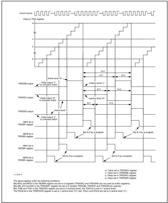
Figure 20.15 Operating Example of PWM Mode
