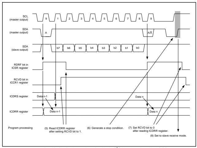
Figure 26.8 Operating Timing in Master Receive Mode (I<sup>2</sup>C bus Interface Mode) (2)
