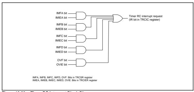
Figure 19.20 Timer RC Interrupt Block Diagram
