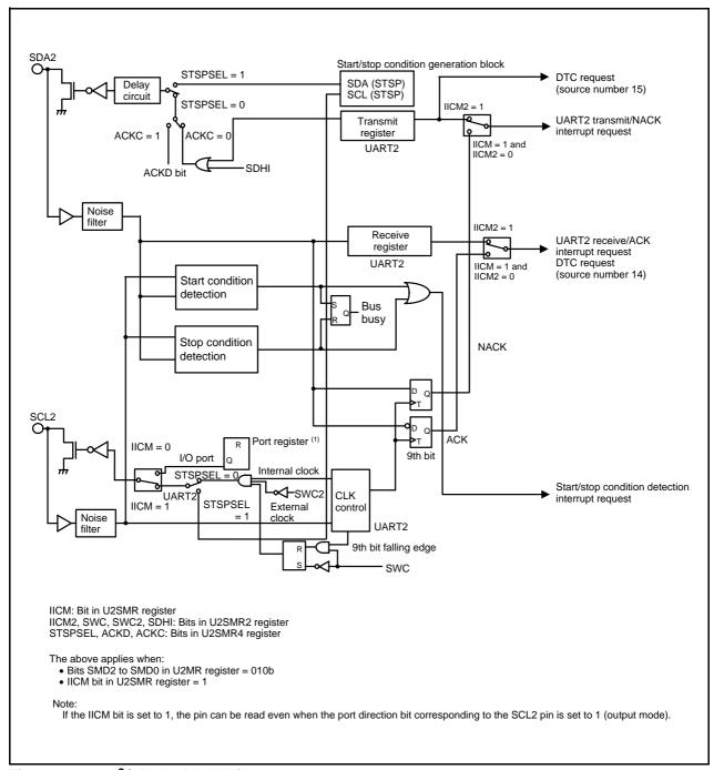
Figure 23.13 I<sup>2</sup>C Mode Block Diagram
