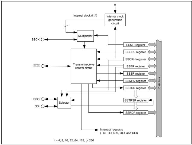
Figure 25.1 Block Diagram of Synchronous Serial Communication Unit
