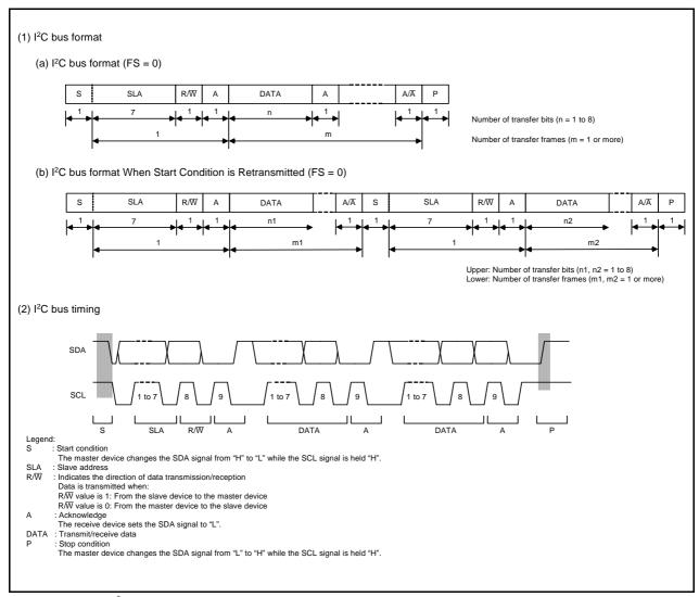
Figure 26.4 I<sup>2</sup>C bus Format and Bus Timing
