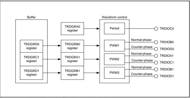
Figure 20.19 Block Diagram of Complementary PWM Mode
