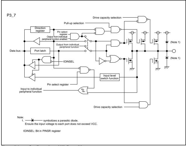
Figure 7.9 Configuration of I/O Ports (9)
