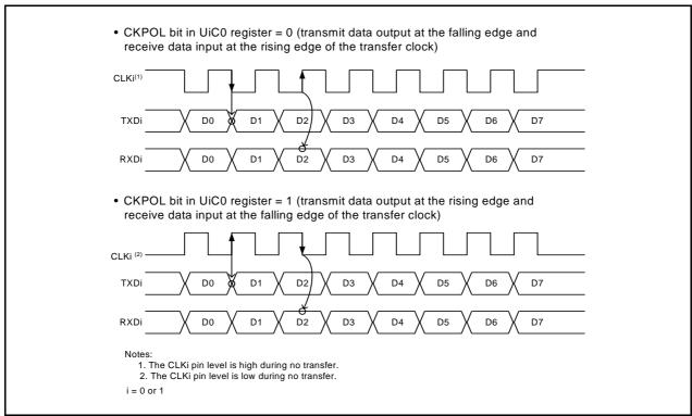
Figure 22.4 Transfer Clock Polarity
