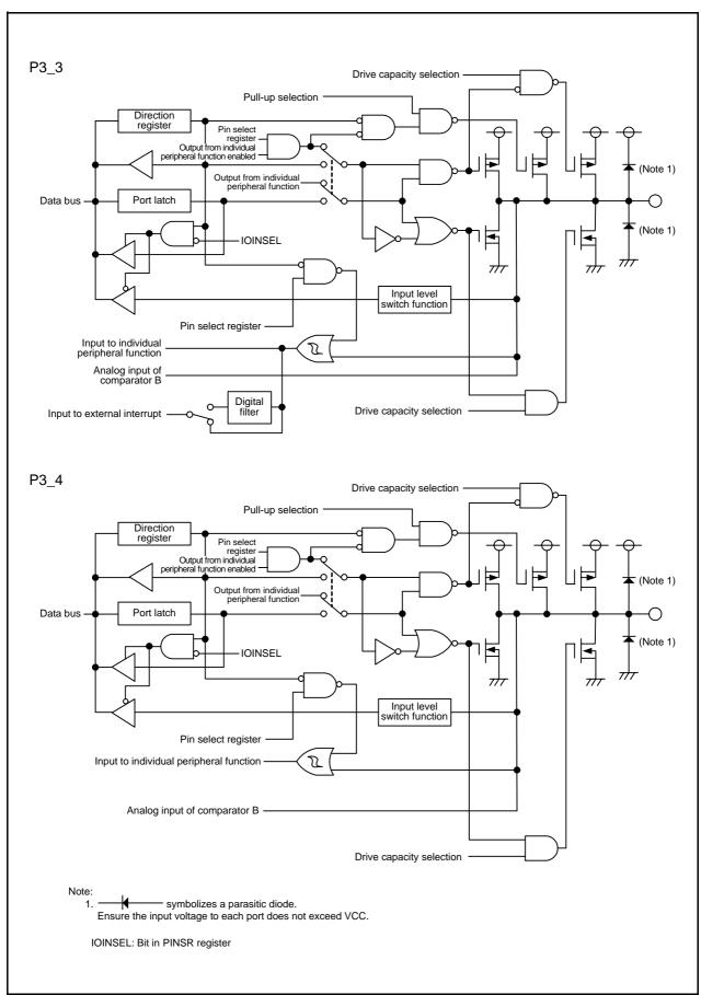
Figure 7.7 Configuration of I/O Ports (7)
