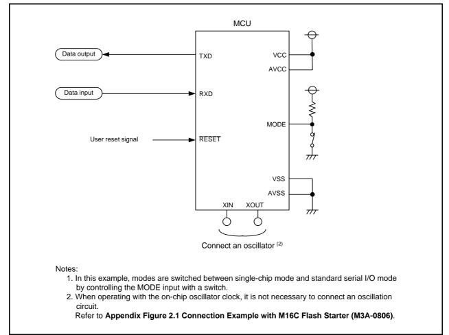
Figure 31.18 Pin Handling in Standard Serial I/O Mode 2
