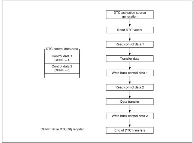
Figure 15.10 Flow of Chain Transfers
