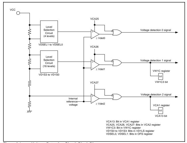
Figure 6.1 Voltage Detection Circuit Block Diagram
