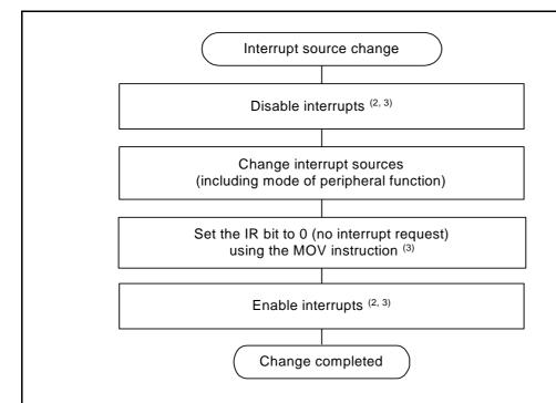
IR bit: The interrupt control register bit for the interrupt whose source is to be changed
