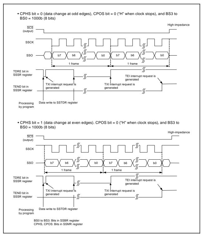
Figure 25.11 Example of Synchronous Serial Communication Unit Operation during Data
