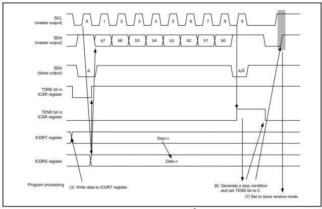
Figure 26.6 Operating Timing in Master Transmit Mode (I<sup>2</sup>C bus Interface Mode) (2)
