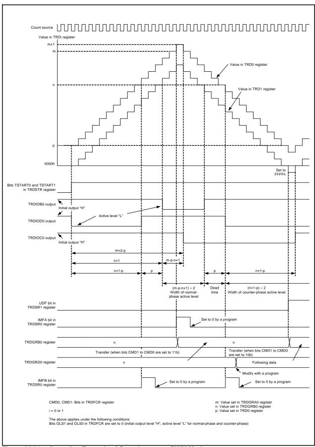
Figure 20.21 Operating Example of Complementary PWM Mode
