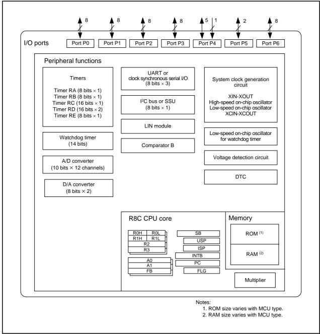
Figure 1.2 Block Diagram
