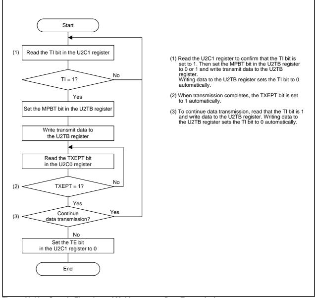
Figure 23.19 Sample Flowchart of Multiprocessor Data Transmission
