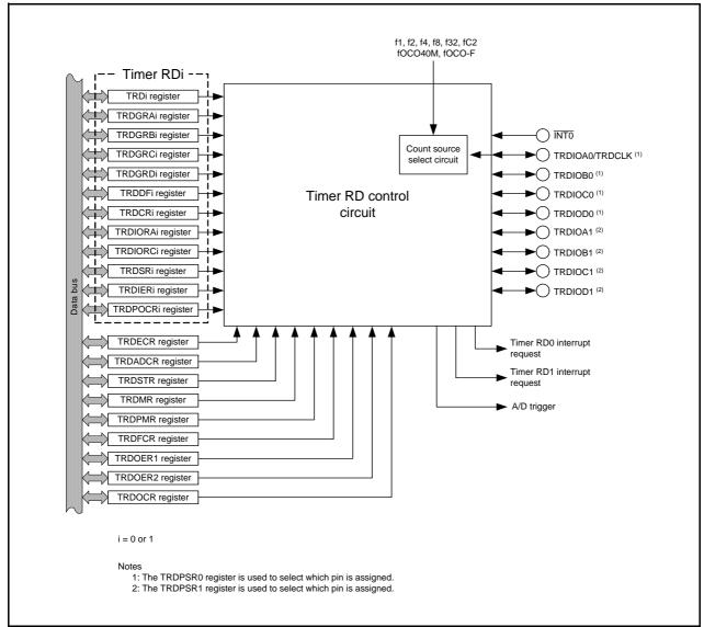
Figure 20.1 Timer RD Block Diagram
