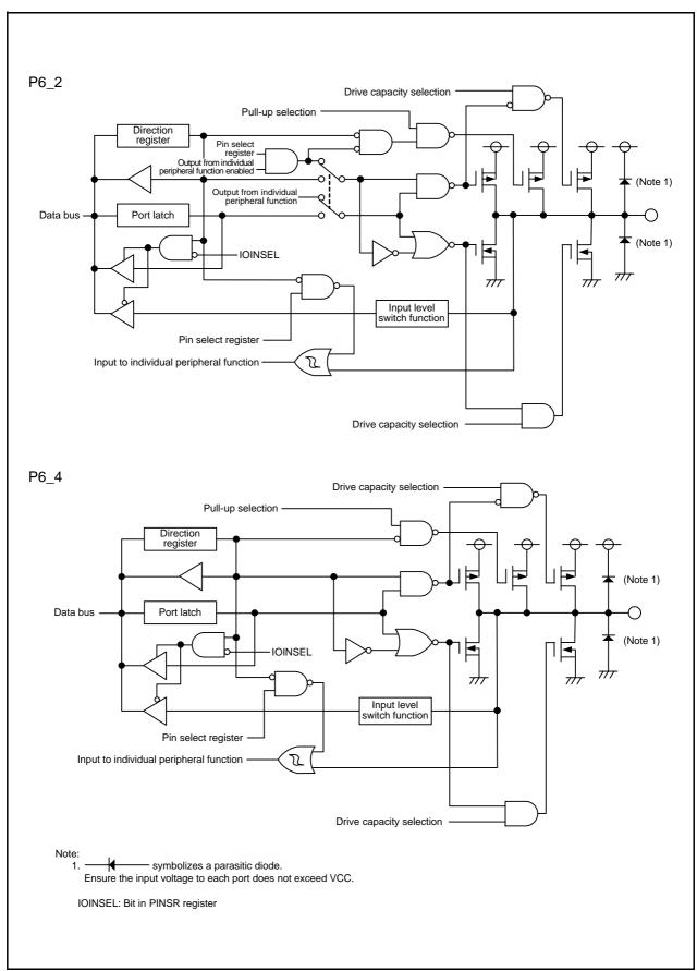
Figure 7.15 Configuration of I/O Ports (15)
