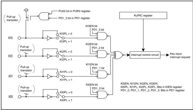
Figure 11.11 Block Diagram of Key Input Interrupt
