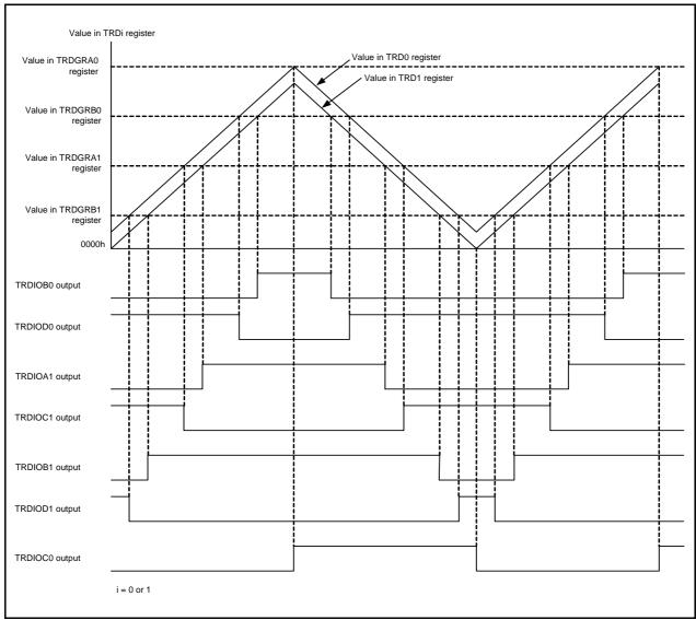
Figure 20.20 Output Model of Complementary PWM Mode
