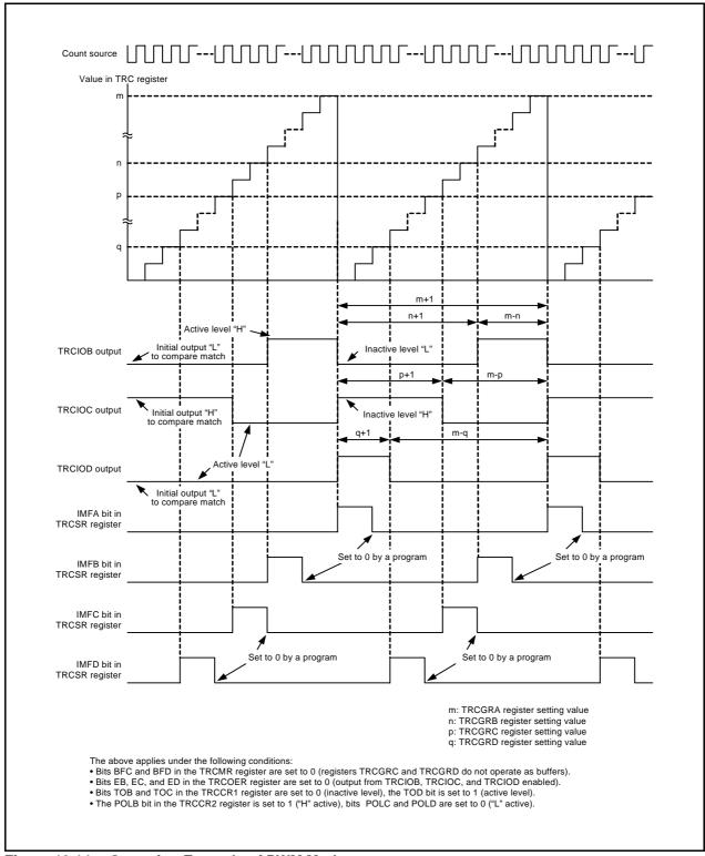
Figure 19.14 Operating Example of PWM Mode
