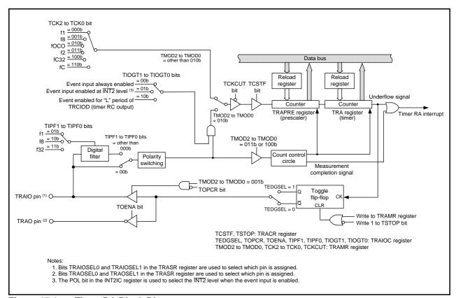
Figure 17.1 Timer RA Block Diagram
