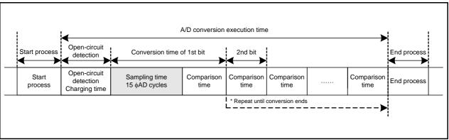
Figure 28.2 Timing Diagram of A/D Conversion
