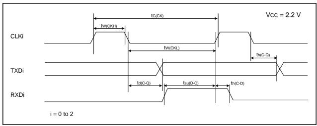
Figure 33.18 Serial Interface Timing Diagram when Vcc = 2.2 V
