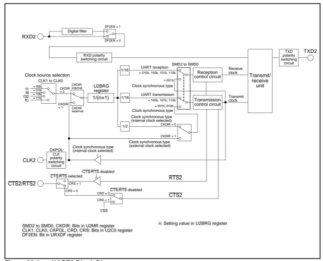
Figure 23.1 UART2 Block Diagram
