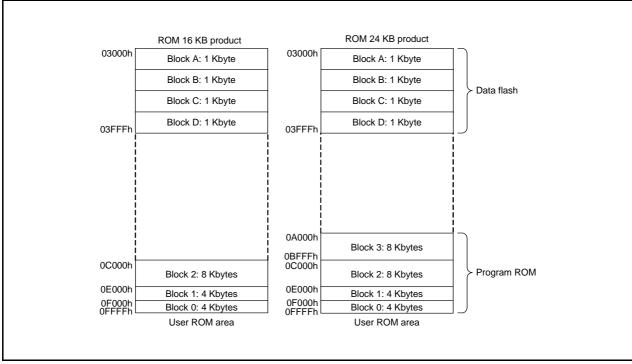
Figure 31.1 R8C/35C Group Flash Memory Block Diagram (1)
