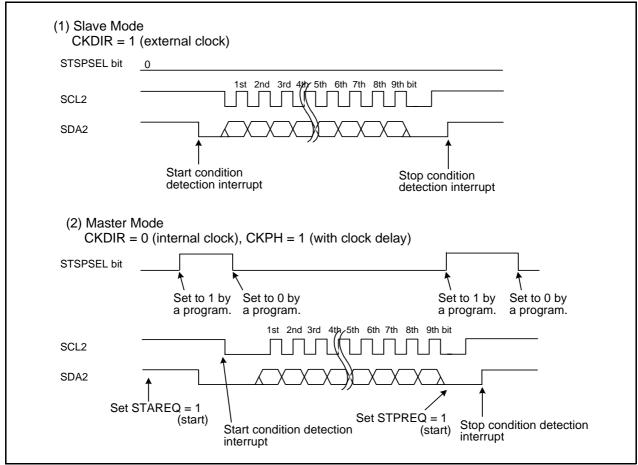
Figure 23.16 STSPSEL Bit Functions
