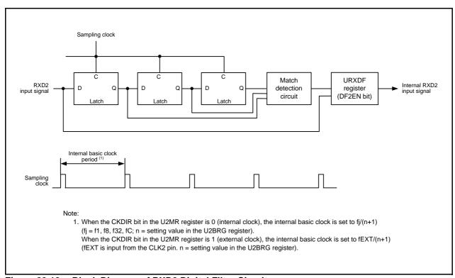
Figure 23.12 Block Diagram of RXD2 Digital Filter Circuit
