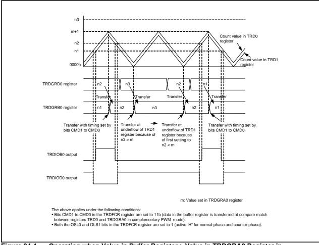
Figure 34.4 Operation when Value in Buffer Register ≥ Value in TRDGRA0 Register in Complementary PWM Mode
