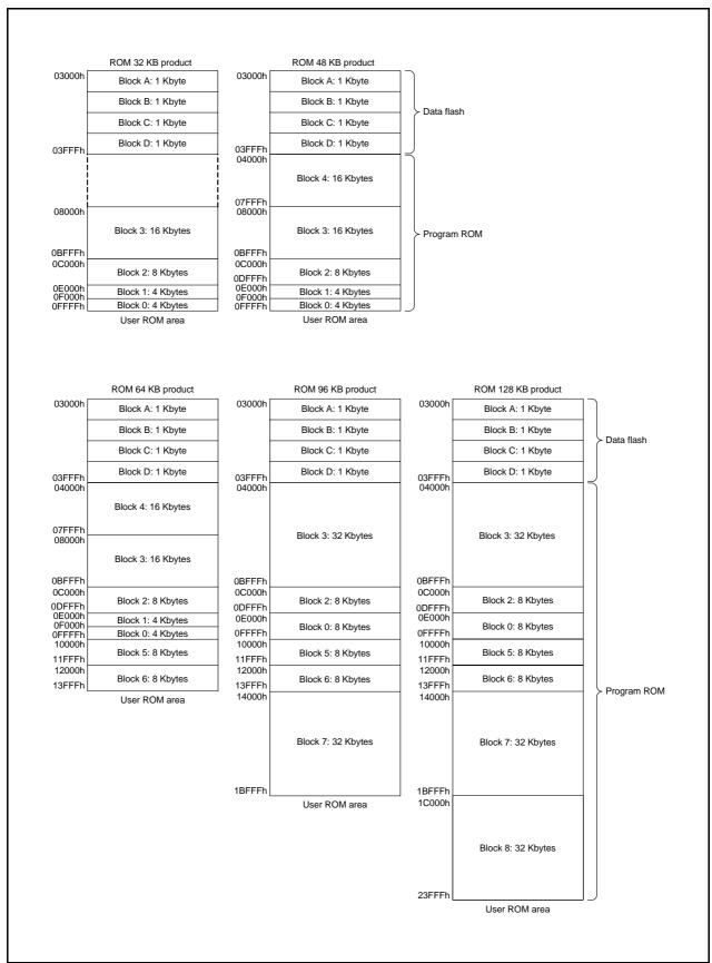
Figure 31.2 R8C/35C Group Flash Memory Block Diagram (2)
