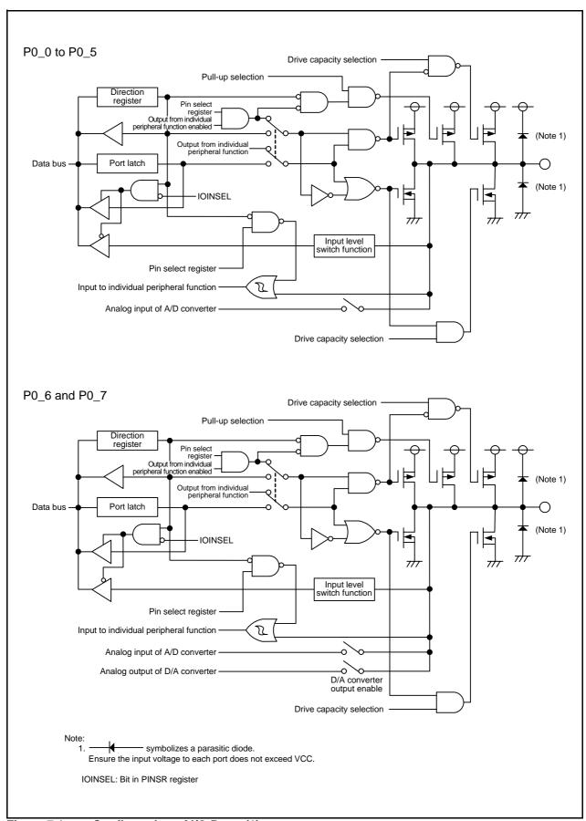
Figure 7.1 Configuration of I/O Ports (1)
