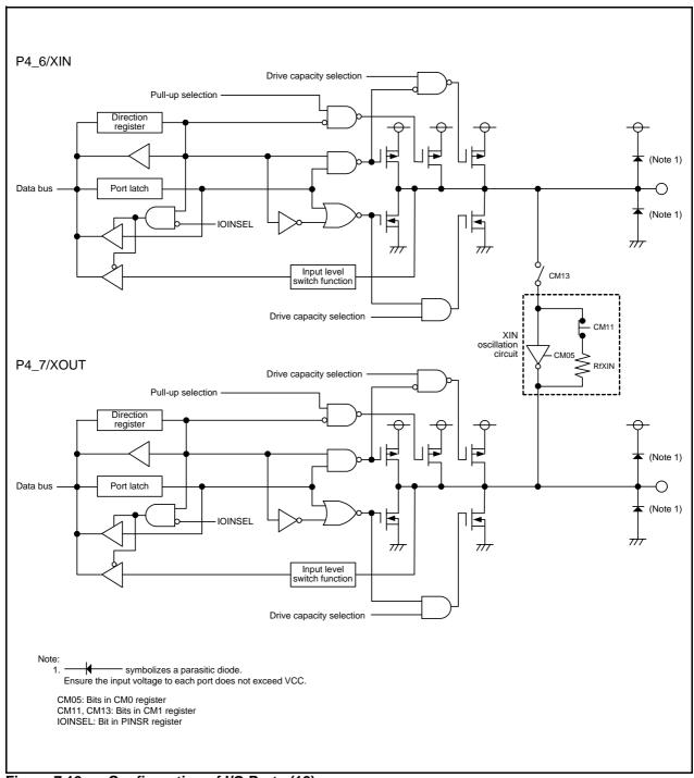
Figure 7.12 Configuration of I/O Ports (12)
