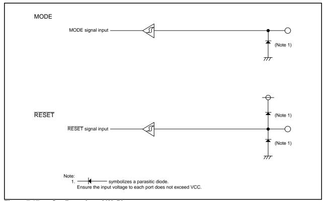
Figure 7.17 Configuration of I/O Pins
