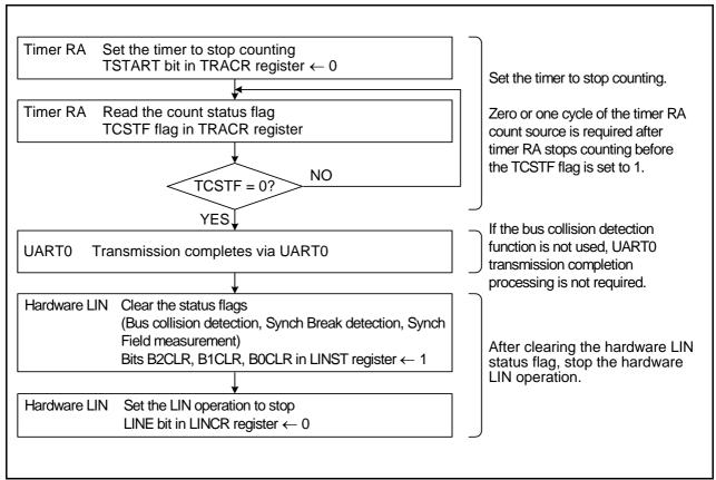
Figure 27.10 Example of Hardware LIN Communication Completion Flowchart
