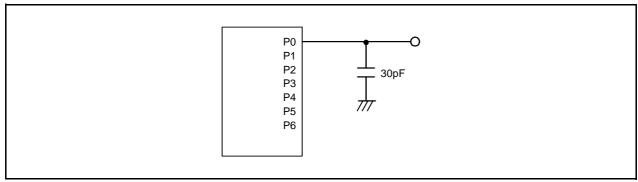
Figure 33.1 Ports P0 to P6 Timing Measurement Circuit
