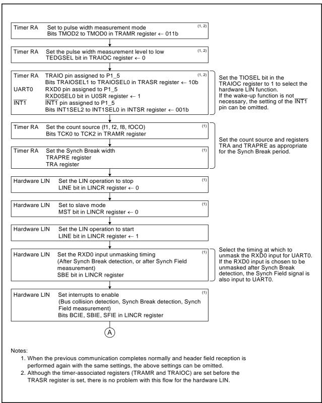
Figure 27.6 Header Field Reception Flowchart Example (1)
