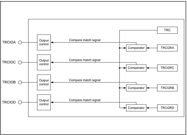
Figure 19.9 Block Diagram of Output Compare Function
