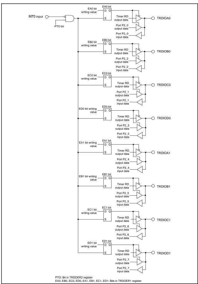
Figure 20.6 Pulse Output Forced Cutoff
