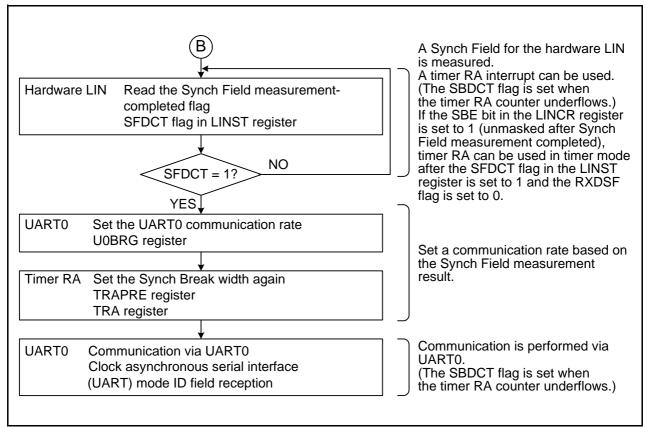
Figure 27.8 Header Field Reception Flowchart Example (3)
