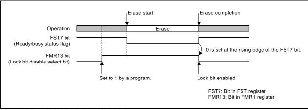
Figure 31.8 FMR13 Bit Operation Timing
