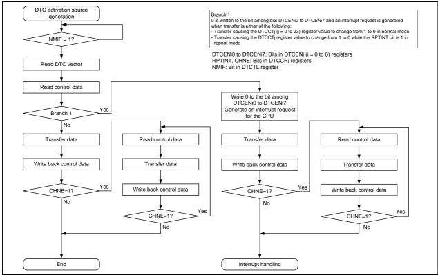
Figure 15.3 DTC Internal Operation Flowchart When DTC Activation Source is not SSU/I<sup>2</sup>C bus, Timer RC, Timer RD, or Flash Memory Interrupt Source
