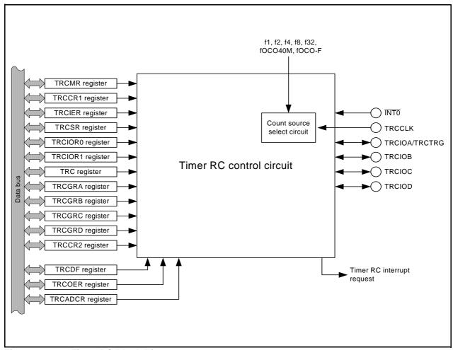
Figure 19.1 Timer RC Block Diagram
