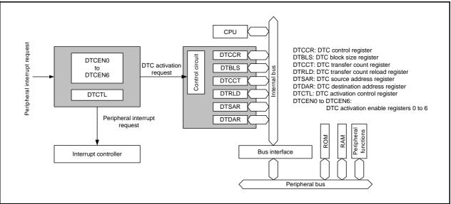
Figure 15.1 DTC Block Diagram
