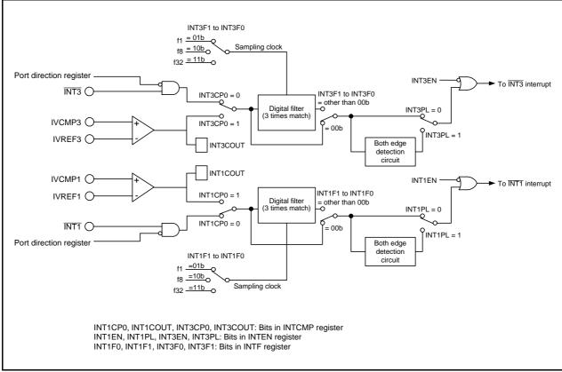
Figure 30.1 Comparator B Block Diagram
