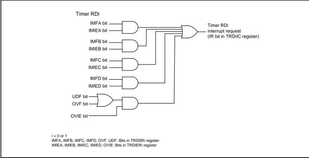
Figure 11.12 Block Diagram of Timer RD Interrupt
