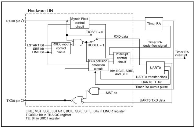
Figure 27.1 Hardware LIN Block Diagram
