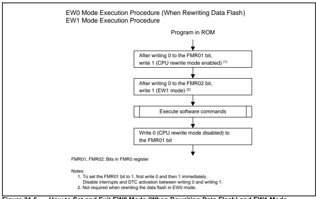
Figure 31.6 How to Set and Exit EW0 Mode (When Rewriting Data Flash) and EW1 Mode
