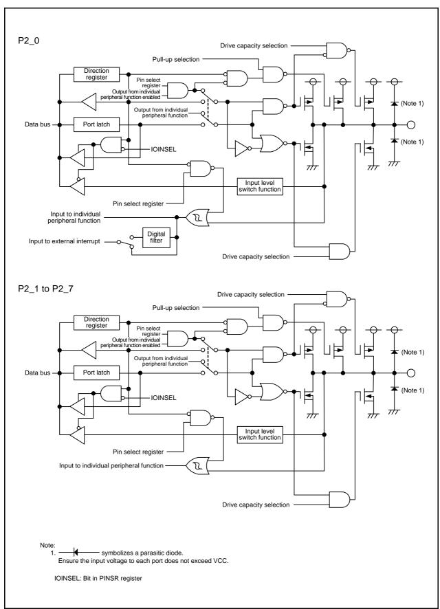
Figure 7.5 Configuration of I/O Ports (5)
