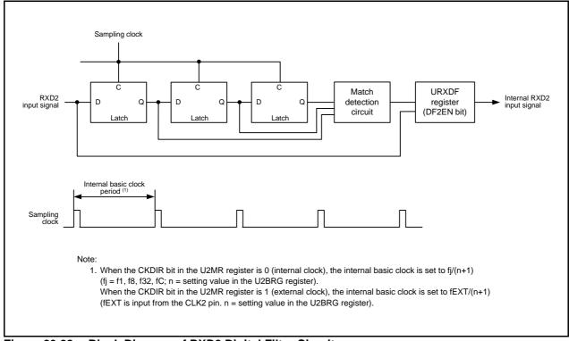
Figure 23.22 Block Diagram of RXD2 Digital Filter Circuit
