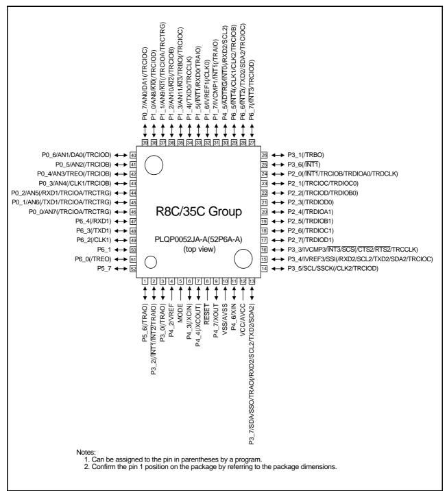
Figure 1.3 Pin Assignment (Top View)
