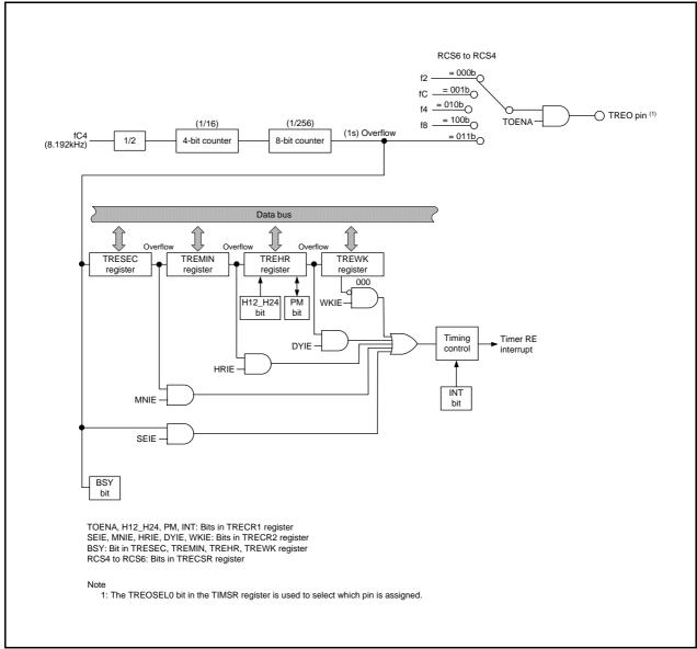
Figure 21.1 Block Diagram of Real-Time Clock Mode
