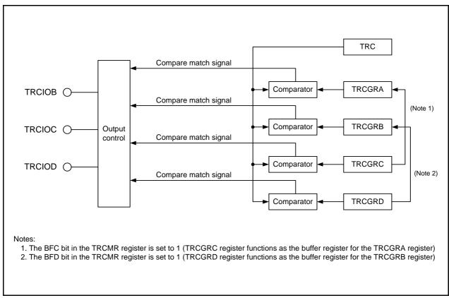
Figure 19.13 PWM Mode Block Diagram
