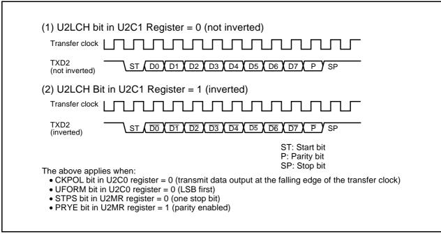
Figure 23.10 Serial Data Logic Switching
