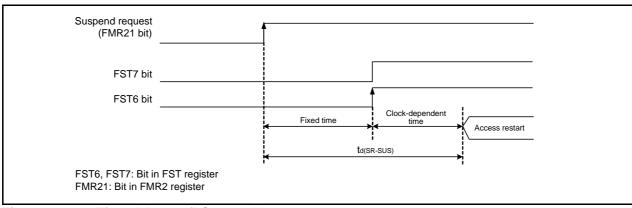
Figure 33.2 Time delay until Suspend
