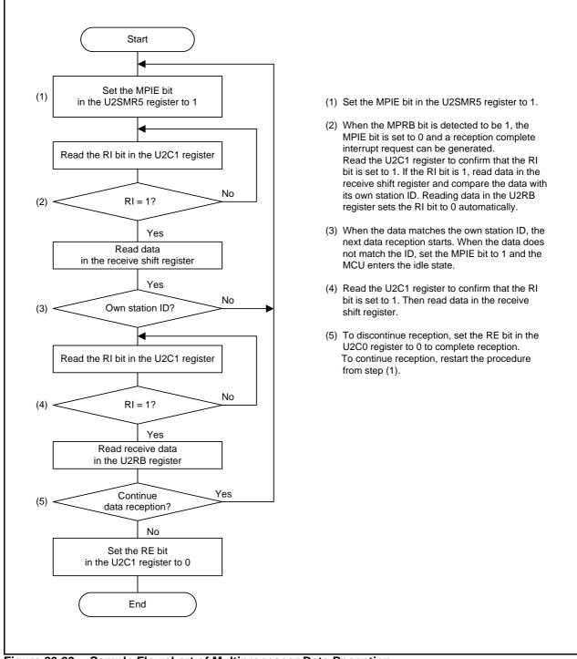
Figure 23.20 Sample Flowchart of Multiprocessor Data Reception
