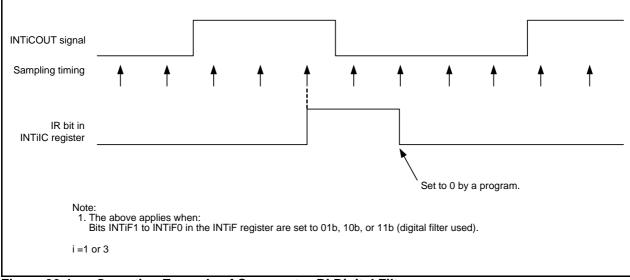
Figure 30.4 Operating Example of Comparator Bi Digital Filter
