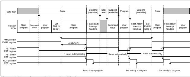
Figure 31.4 **Suspend Operation Timing**
