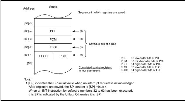
Figure 11.6 Register Saving Operation
