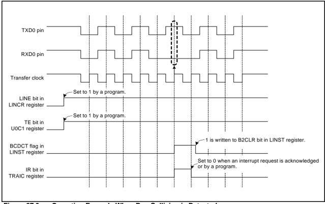
Figure 27.9 Operating Example When Bus Collision is Detected
