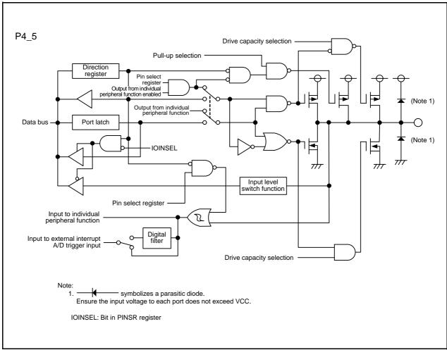
Figure 7.11 Configuration of I/O Ports (11)
