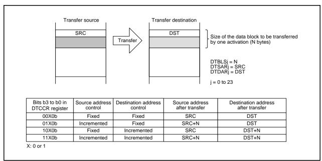
Figure 15.8 Data Transfers in Normal Mode
