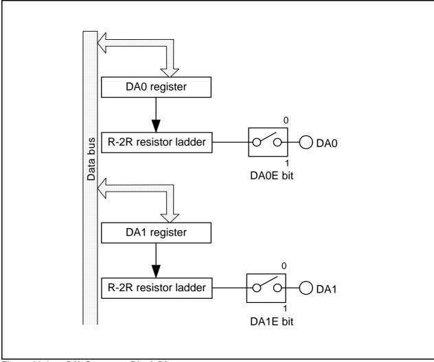
Figure 29.1 D/A Converter Block Diagram
