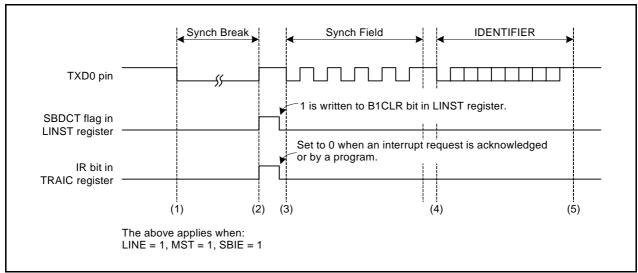
Figure 27.2 Operating Example during Header Field Transmission
