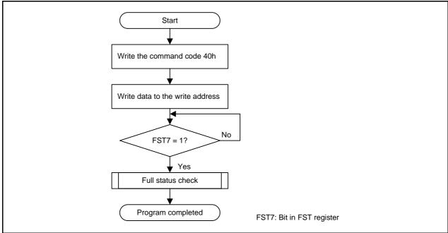
Figure 31.9 Program Flowchart (Flash Ready Status Interrupt Disabled)
