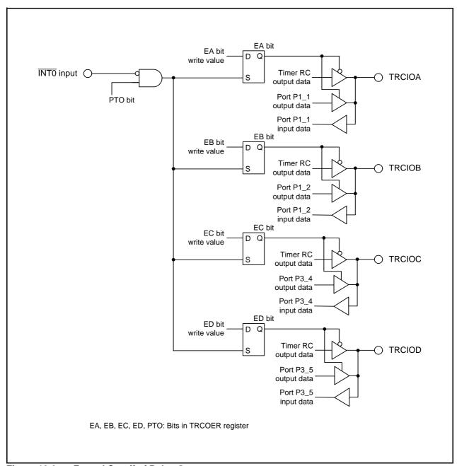
Figure 19.6 Forced Cutoff of Pulse Output
