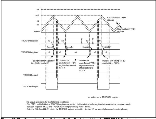
Figure 20.27 Operation when Value in Buffer Register ≥ Value in TRDGRA0 Register in Complementary PWM Mode
