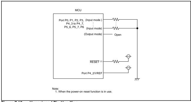
Figure 7.18 Unassigned Pin Handling
