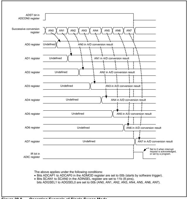
Figure 28.8 Operating Example of Single Sweep Mode
