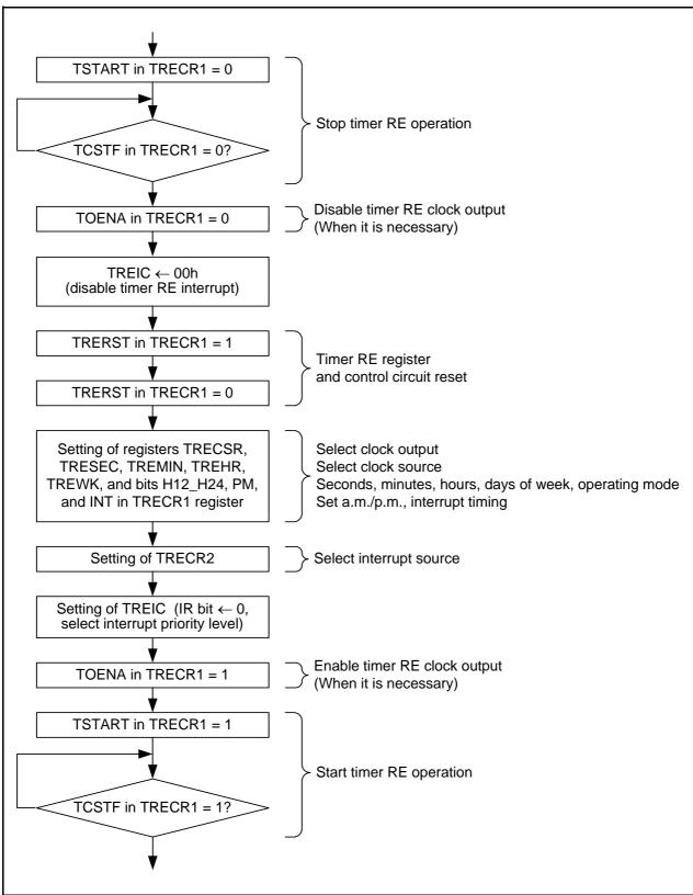
Figure 34.6 Setting Example in Real-Time Clock Mode
