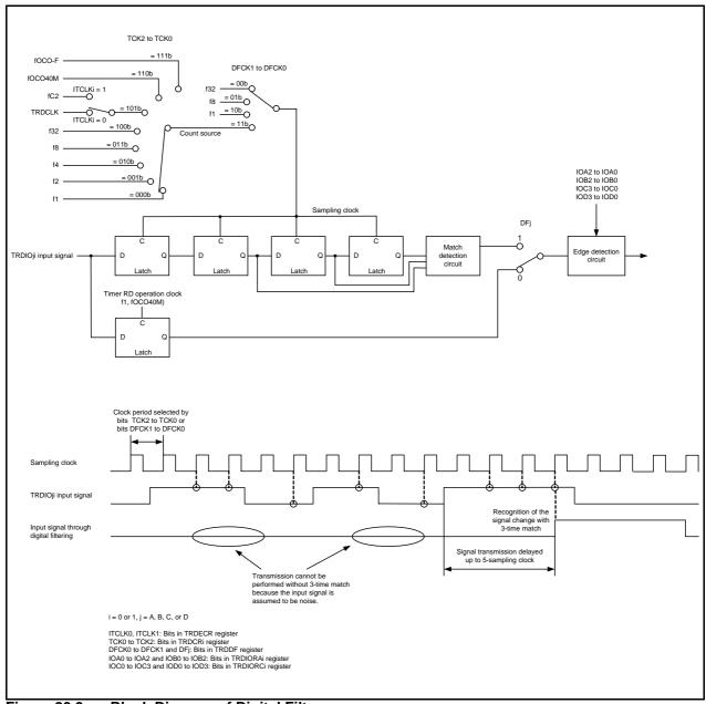
Figure 20.9 Block Diagram of Digital Filter
