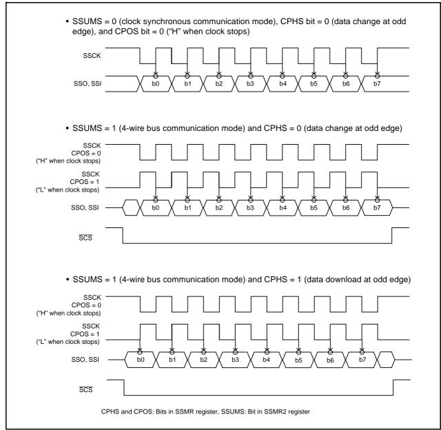
Figure 25.2 Association between Transfer Clock Polarity, Phase, and Transfer Data
