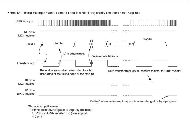
Figure 22.7 Receive Timing in UART Mode
