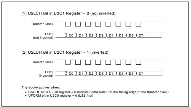
Figure 23.6 Serial Data Logic Switching
