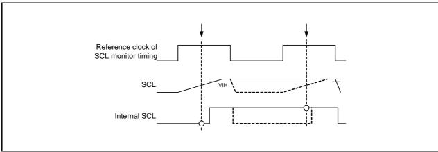
Figure 26.21 Bit Synchronization Circuit Timing
