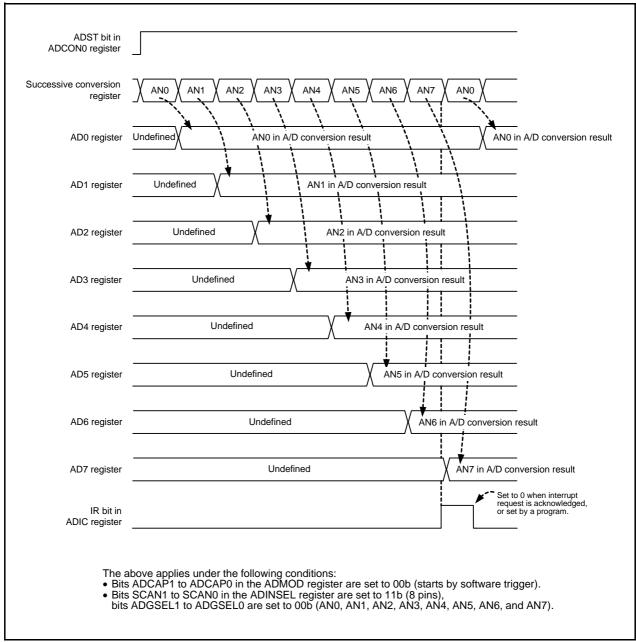
Figure 28.9 Operating Example of Repeat Sweep Mode
