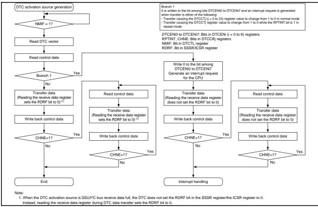
Figure 15.5 DTC Internal Operation Flowchart When DTC Activation Source is SSU/I<sup>2</sup>C bus Receive Data Full
