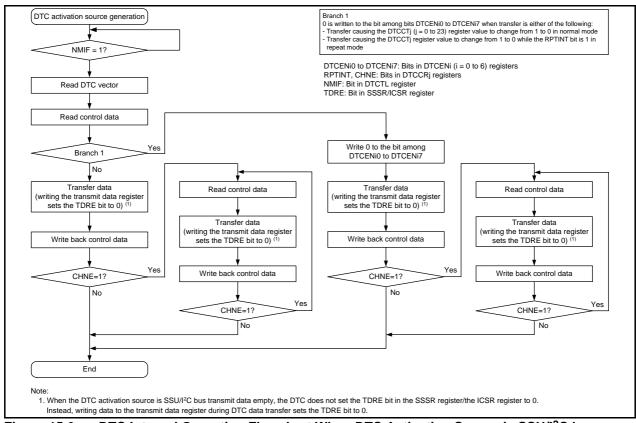
Figure 15.6 DTC Internal Operation Flowchart When DTC Activation Source is SSU/I<sup>2</sup>C bus Transmit Data Empty
