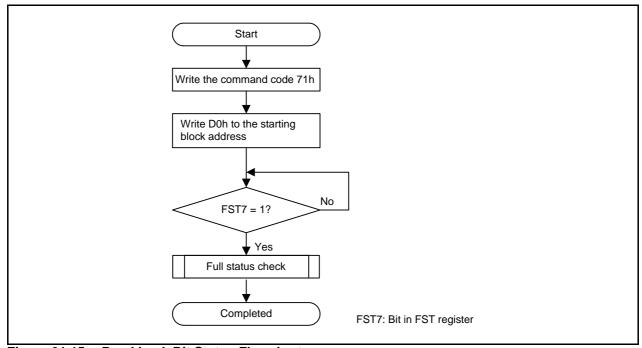
Figure 31.15 Read Lock Bit Status Flowchart
