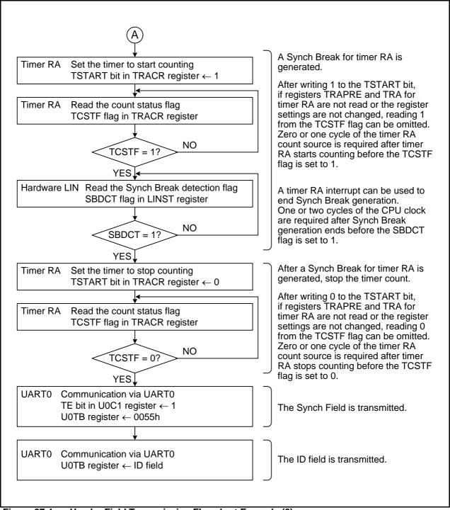
Figure 27.4 Header Field Transmission Flowchart Example (2)
