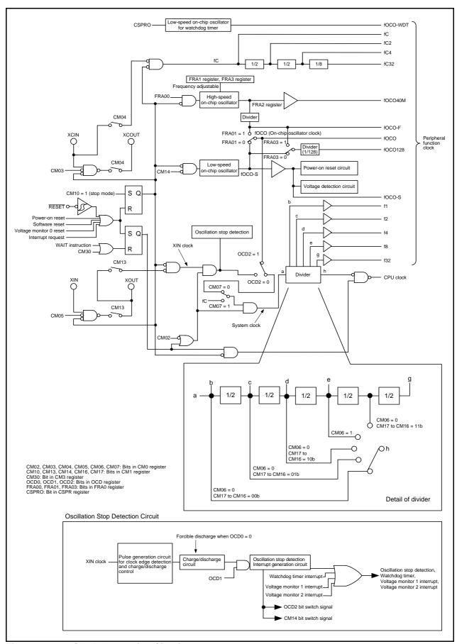
Figure 9.1 Clock Generation Circuit
