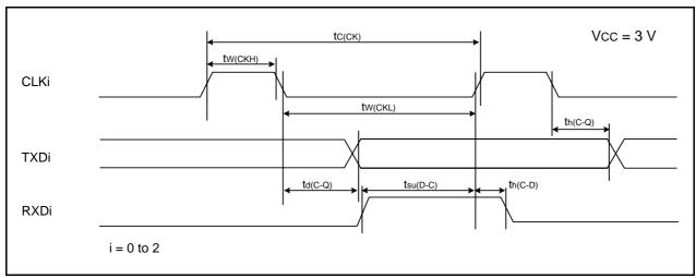
Figure 33.14 Serial Interface Timing Diagram when Vcc = 3 V
