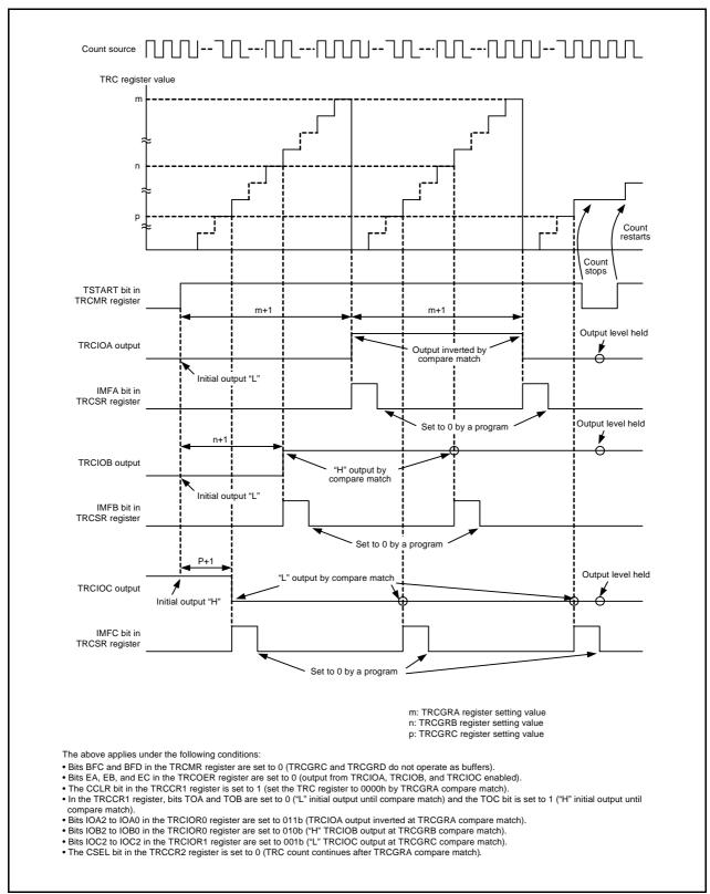
Figure 19.10 Operating Example of Output Compare Function
