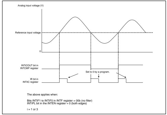
Figure 30.2 Operating Example of Comparator Bi (i = 1 or 3)
