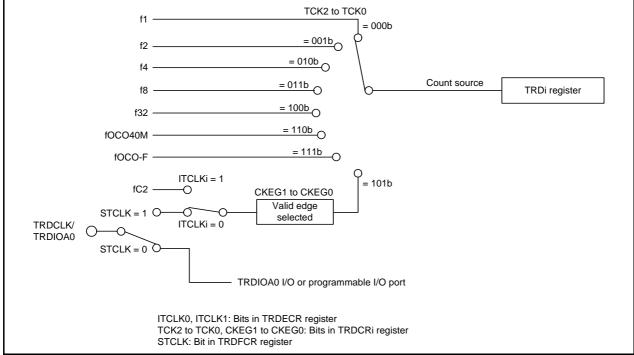
Figure 20.2 Block Diagram of Count Source
