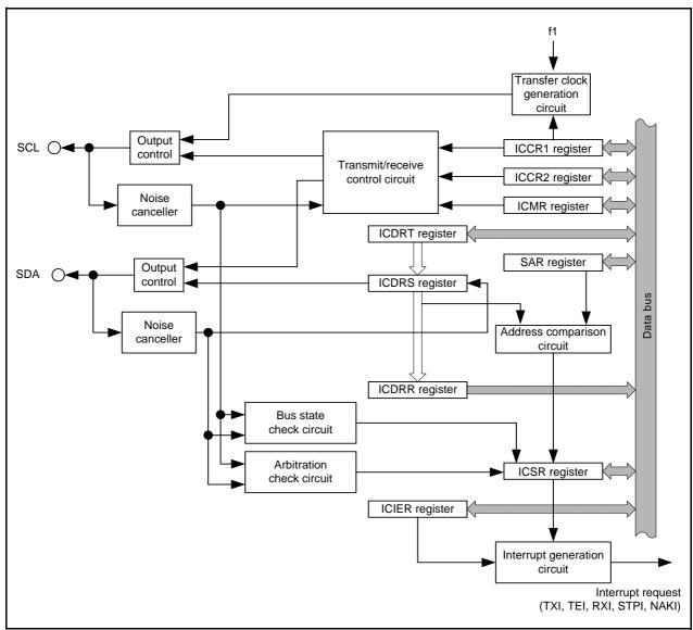
Figure 26.1 I<sup>2</sup>C bus interface Block Diagram
