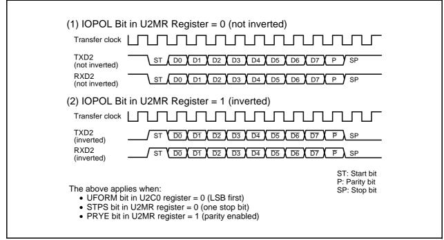
Figure 23.11 TXD and RXD I/O Inversion
