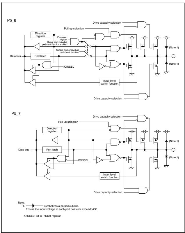
Figure 7.13 Configuration of I/O Ports (13)
