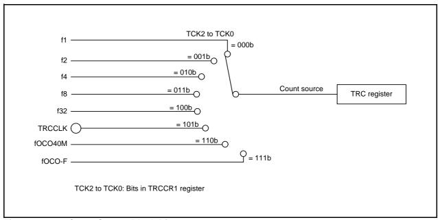
Figure 19.2 Count Source Block Diagram
