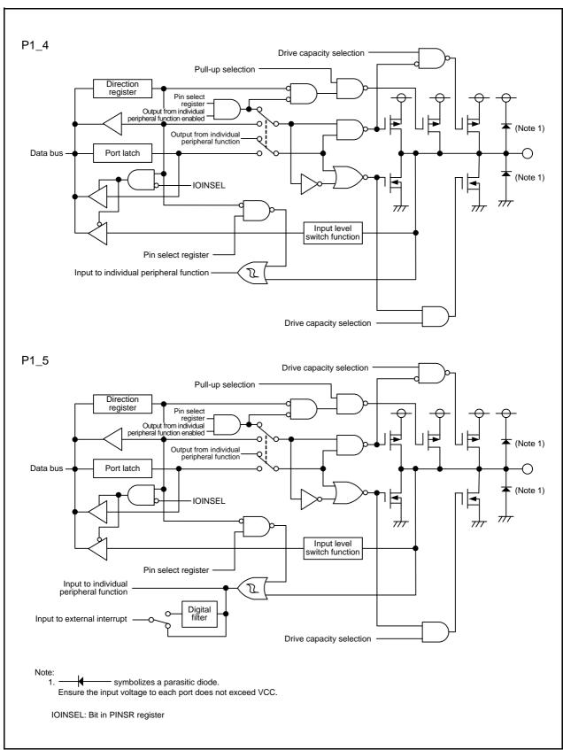
Figure 7.3 Configuration of I/O Ports (3)
