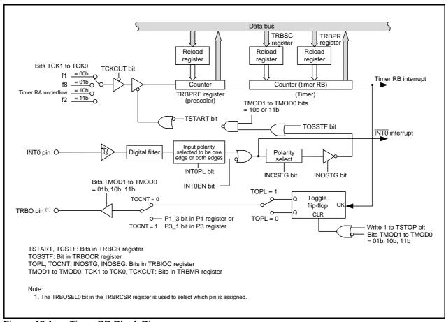
Figure 18.1 Timer RB Block Diagram
