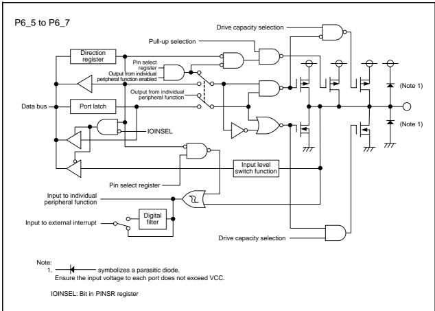
Figure 7.16 Configuration of I/O Ports (16)
