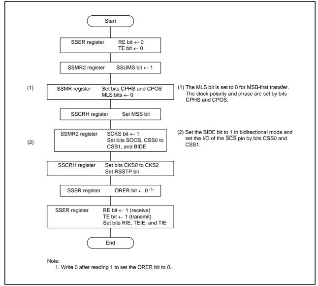
Figure 25.10 Initialization in 4-Wire Bus Communication Mode
