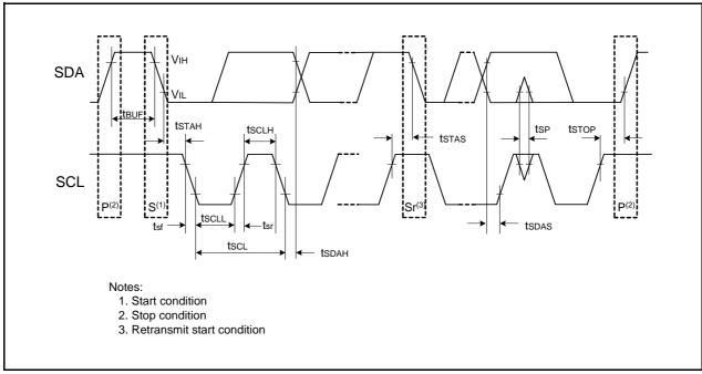
Figure 33.7 I/O Timing of I<sup>2</sup>C bus Interface
