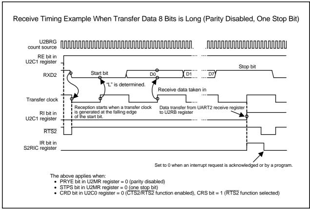
Figure 23.8 Receive Timing in UART Mode
