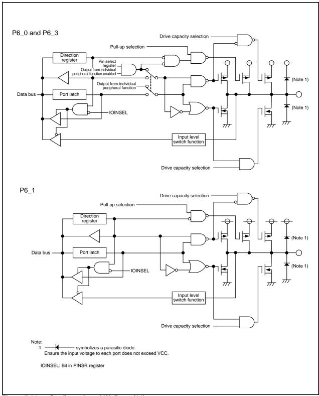
Figure 7.14 Configuration of I/O Ports (14)
