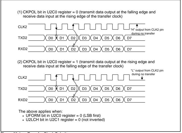
Figure 23.4 Transfer Clock Polarity
