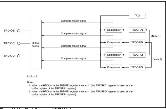
Figure 20.14 Block Diagram of PWM Mode
