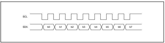
Figure 26.13 Transfer Format of Clock Synchronous Serial Format
