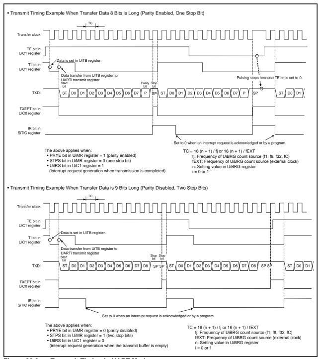
Figure 22.6 Transmit Timing in UART Mode
