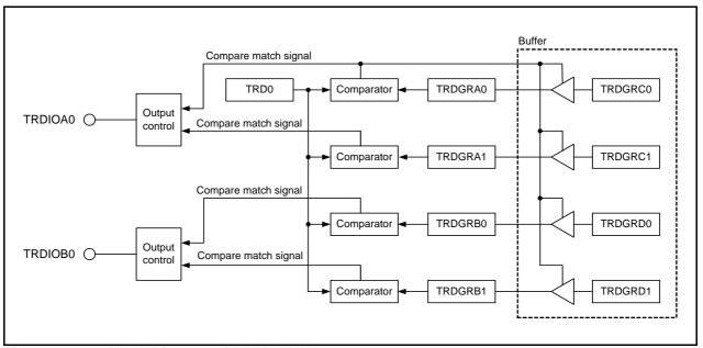
Figure 20.22 Block Diagram of PWM3 Mode
