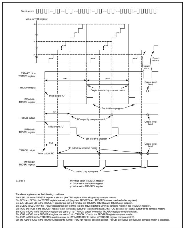
Figure 20.11 Operating Example of Output Compare Function
