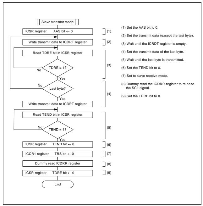
Figure 26.18 Register Setting Example in Slave Transmit Mode (I<sup>2</sup>C bus Interface Mode)
