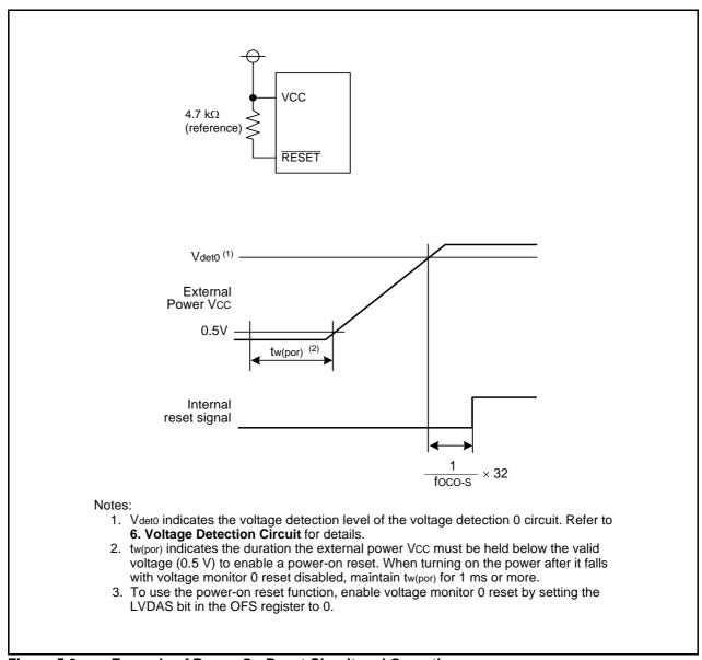
Figure 5.6 Example of Power-On Reset Circuit and Operation
