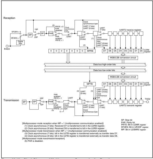
Figure 23.18 Block Diagram of Multiprocessor Communication Function
