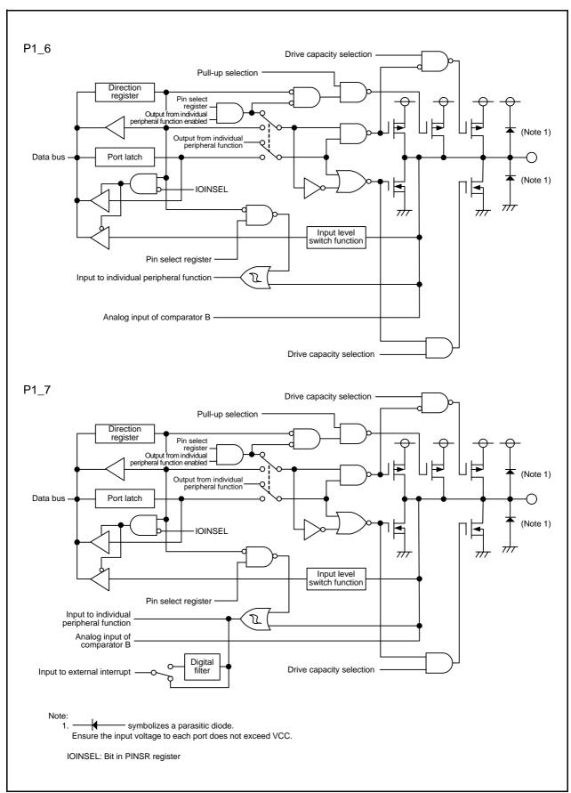
Figure 7.4 Configuration of I/O Ports (4)
