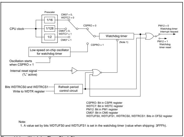
Figure 14.1 Watchdog Timer Block Diagram
