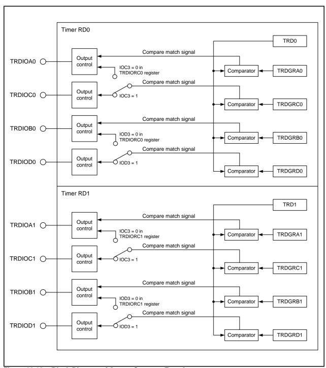
Figure 20.10 Block Diagram of Output Compare Function
