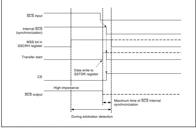
Figure 25.13 Arbitration Check Timing
