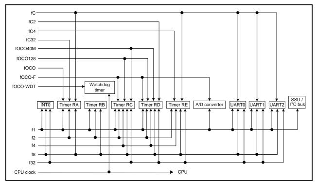
Figure 9.2 Peripheral Function Clock
