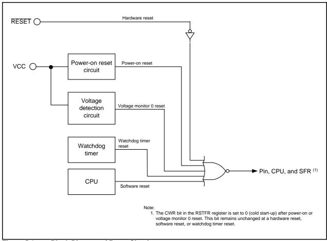
Figure 5.1 Block Diagram of Reset Circuit
