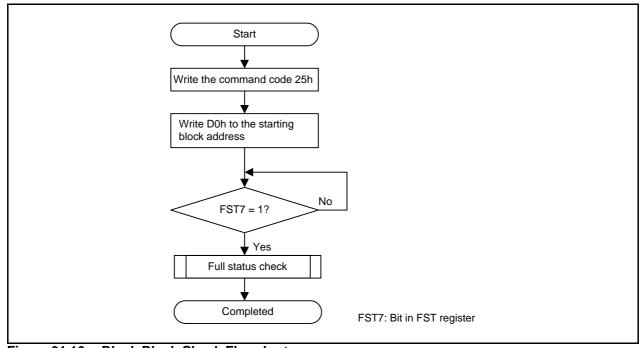
Figure 31.16 Block Blank Check Flowchart
