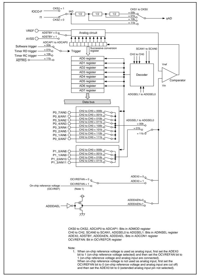
Figure 28.1 Block Diagram of A/D Converter
