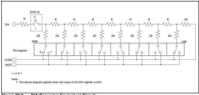
Figure 29.2 D/A Converter Equivalent Circuit
