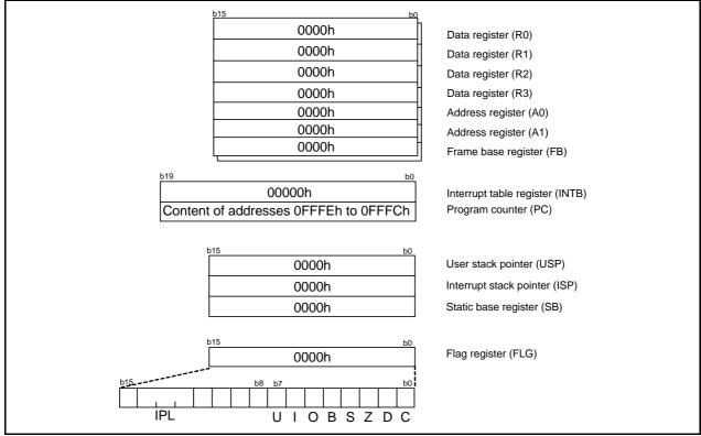
Figure 5.2 CPU Register Status after Reset
