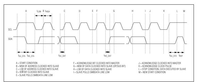
Figure 8. I<sup>2</sup>C Timing Diagram
