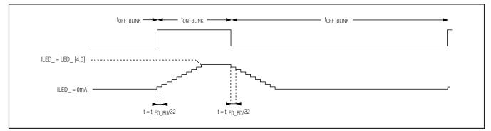
Figure 6. Combining Ramp Function and Blink Timer (Tables 10 and 11)
