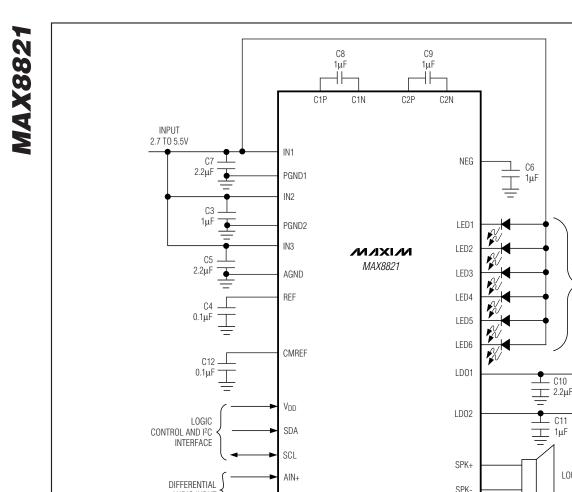
Figure 2. Typical Application Circuit
