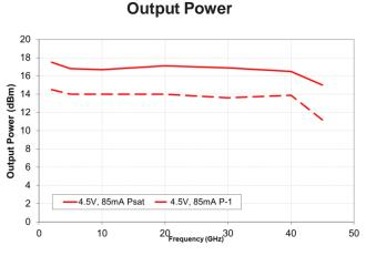
Typical IC performance measured on-wafer
