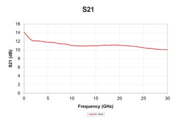
Typical IC performance measured on-wafer
