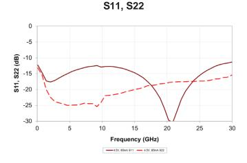
Typical IC performance measured on-wafer
