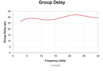
Typical IC performance measured on-wafer
