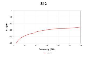
Typical IC performance measured on-wafer
