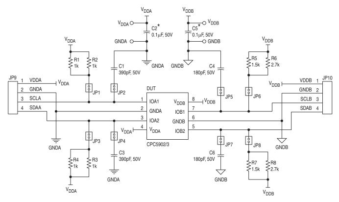
\*Note: C2 and C5 are located on the bottom side of the board
