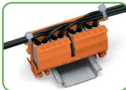
Strain relief by cable tie on the carrier, transverse to the connectors wiring direction. Molded marking of clamping units.
