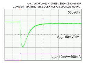
$\begin{array}{c} \text{XC9246B} \\ \text{V}_{\text{IN}}\text{=}12\text{V}, \, \text{V}_{\text{OUT}}\text{=}3.3\text{V}, \, \text{I}_{\text{OUT}}\text{=}500\text{mA} \rightarrow 10\text{mA} \end{array}$
