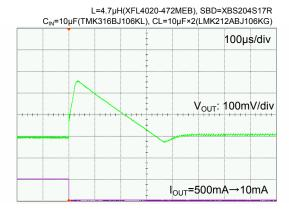
$\begin{tabular}{ll} $XC9247B$ \\ $V_{IN}$=$12V, $V_{OUT}$=$3.3V, $I_{OUT}$=$200mA$$\rightarrow$800mA$ \\ \end{tabular}$
