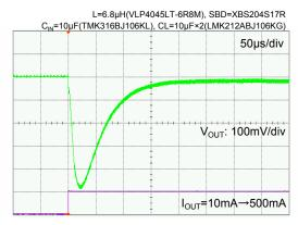
XC9247B VIN=12V, VOUT=5.0V, IOUT=500mA→10mA
