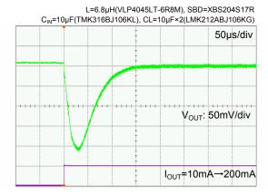
XC9246B VIN=12V, VOUT=5.0V, IOUT=200mA→10mA
