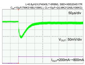
XC9246B VIN=12V, VOUT=5.0V, IOUT=800mA→200mA
