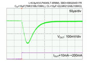
XC9247B VIN=12V, VOUT=5.0V, IOUT=200mA→10mA
