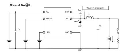
\* External components  $C_{Dic}$ :10  $\mu$  F(ceramic)  $C_{L}$ :22  $\mu$  F(ceramic)  $C_{BST}$ :0.22  $\mu$  F(ceramic) L:4.7  $\mu$  H SBD:XBS204S17R-G
