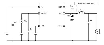
\*External components  $C_{\rm BH}$ 10  $\mu$  F(ceramic)  $C_{\rm L}$ :22  $\mu$  F(ceramic)  $C_{\rm BST}$ 0.22  $\mu$  F(ceramic) L:4.7  $\mu$ H SBD:XBS:204S17R-G  $R_{\rm SS}$ 120k  $\Omega$   $C_{\rm SS}$ 0.47  $\mu$ F
