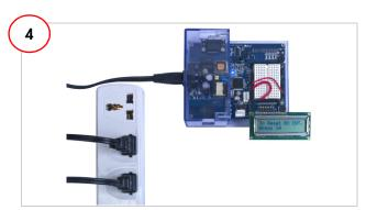
1. Connect the power cable from the AC mains to the AC power connector on the first CY3274 kit. The blue LED (DS1) turns on. Repeat the same for kit 2.
