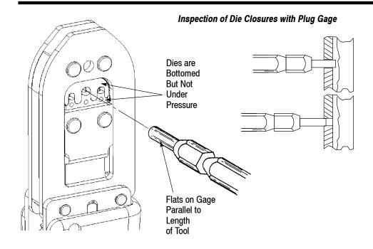
"GO" element must pass completely through the die closure.
