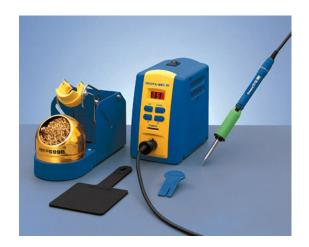
sleep mode of 0-29 minutes or auto-power shut off at 30 minutes. The sleep mode reduces the tip temperature to approximately 200°C (400°F) after the programmed time (0-29 minutes). The lower tip temperature will reduce oxidation of the tip and improve the tip performance. When in sleep mode the tip will quickly return to temperature after the iron is removed from the holder.
