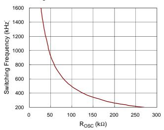
Figure 7. Switching Frequency vs. Rosc Resistor
