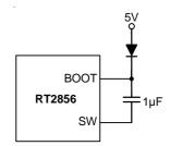
Figure 9. External Bootstrap Diode
