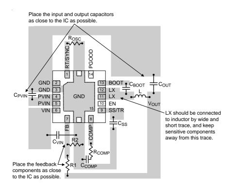
Figure 11. PCB Layout Guide
