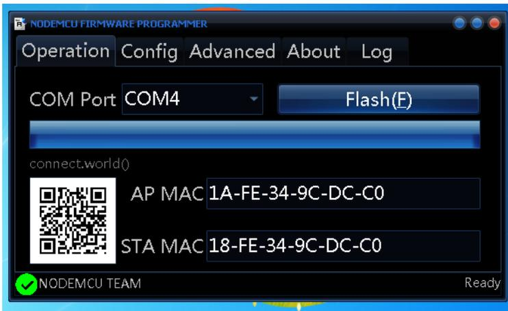
Congratulations, you've loaded the MicroPython firmware on the ESP8266! In the future if you'd like to load the firmware again you can repeat the process above to put the ESP8266 into programming mode and run nodemcu-flasher to upload code.
