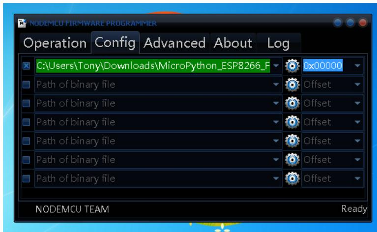
It's very important that your configuration looks like the above with the firmware loaded to offset 0x00000. If you have other firmware files or a different offset then the firmware won't work!
