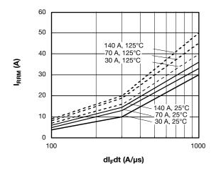
Fig. 6 - Typical Recovery Current vs. dl<sub>F</sub>/dt (Per Leg)
