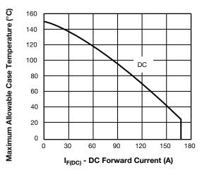
Fig. 4 - Maximum Allowable Case Temperature vs. DC Forward Current (Per Leg)
