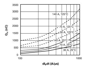
Fig. 7 - Typical Stored Charge vs. dl<sub>F</sub>/dt (Per Leg)
