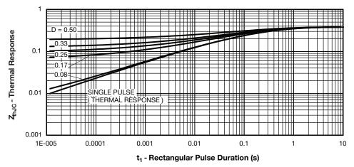
Fig. 9 - Maximum Thermal Impedance  $Z_{thJC}$  Characteristics
