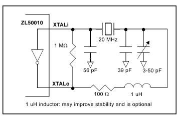
Figure 31 - Crystal Oscillator Circuit
