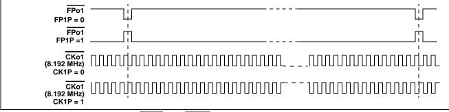
Figure 11 -  $\overline{FP01}$  and  $\overline{CK01}$  Output Timing when the CKFP1 Bit = 1
