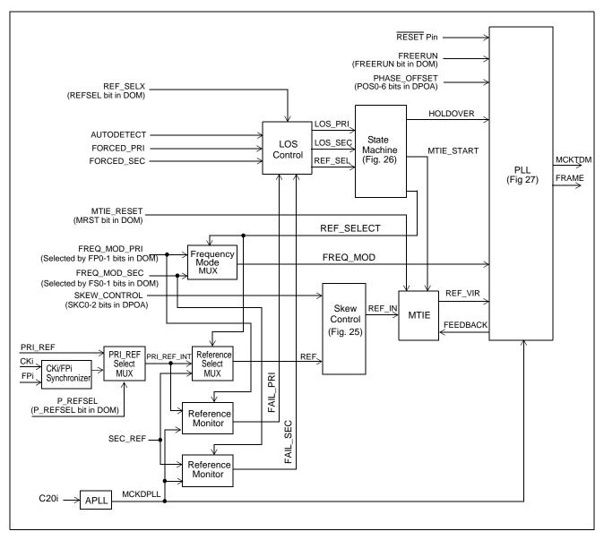
Figure 25 - DPLL Functional Block Diagram
