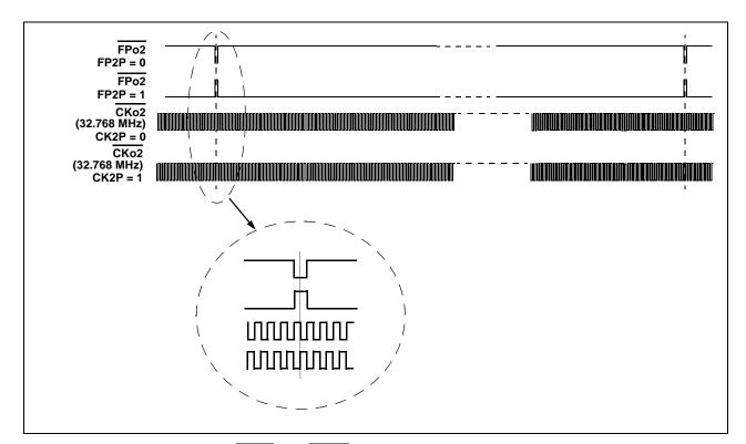
Figure 12 -  $\overline{FPo2}$  and  $\overline{CKo2}$  Output Timing when the CKFP2 Bit = 0
