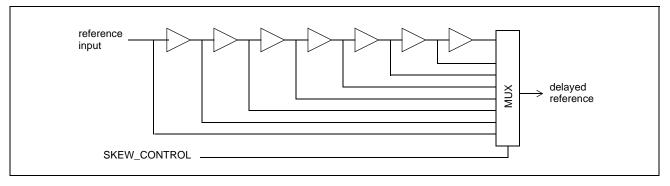
Figure 26 - Skew Control Circuit Diagram
