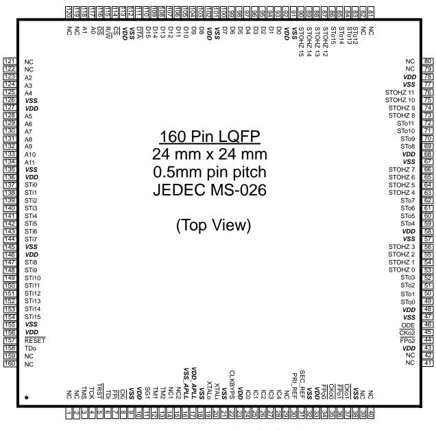
Figure 2 - 24 mm x 24 mm LQFP (JEDEC MS-026) Pinout Diagram
