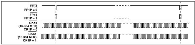
Figure 10 -  $\overline{\text{FPo1}}$  and  $\overline{\text{CKo1}}$  Output Timing when the CKFP1 Bit = 0
