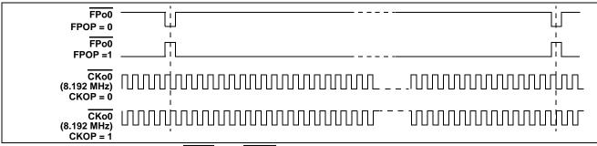
Figure 9 -  $\overline{PPO0}$  and  $\overline{CKo0}$  Output Timing when the CKFP0 Bit = 1
