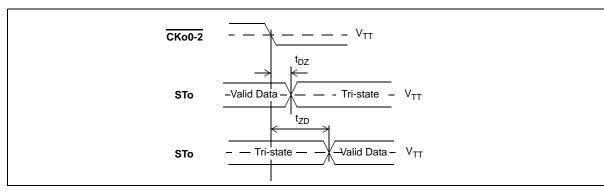
Figure 46 - Serial Output and External Control
