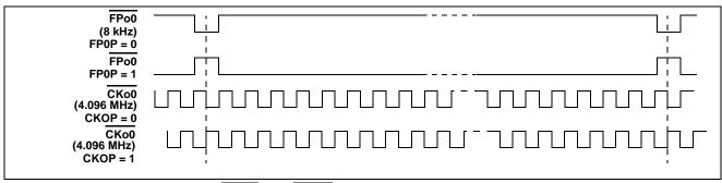
Figure 8 -  $\overline{PPO0}$  and  $\overline{CKo0}$  Output Timing when the CKFP0 Bit = 0
