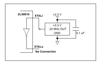
Figure 32 - External Clock Oscillator Circuit
