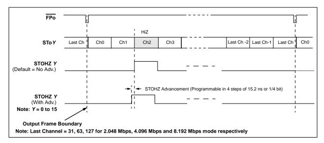
Figure 20 - Example: External High Impedance Control Timing
