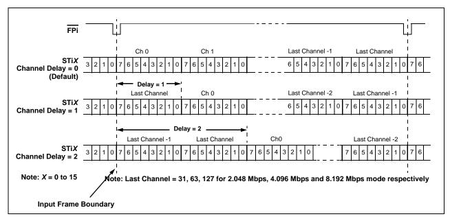
Figure 15 - Input Channel Delay Timing Diagram
