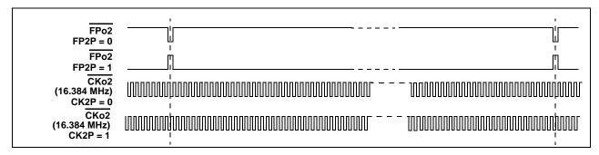
Figure 13 -  $\overline{FPo2}$  and  $\overline{CKo2}$  Output Timing when the CKFP2 Bit = 1
