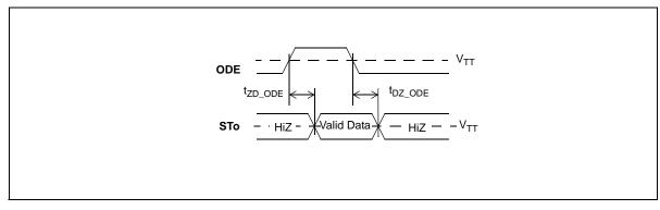
Figure 47 - Output Driver Enable (ODE)
