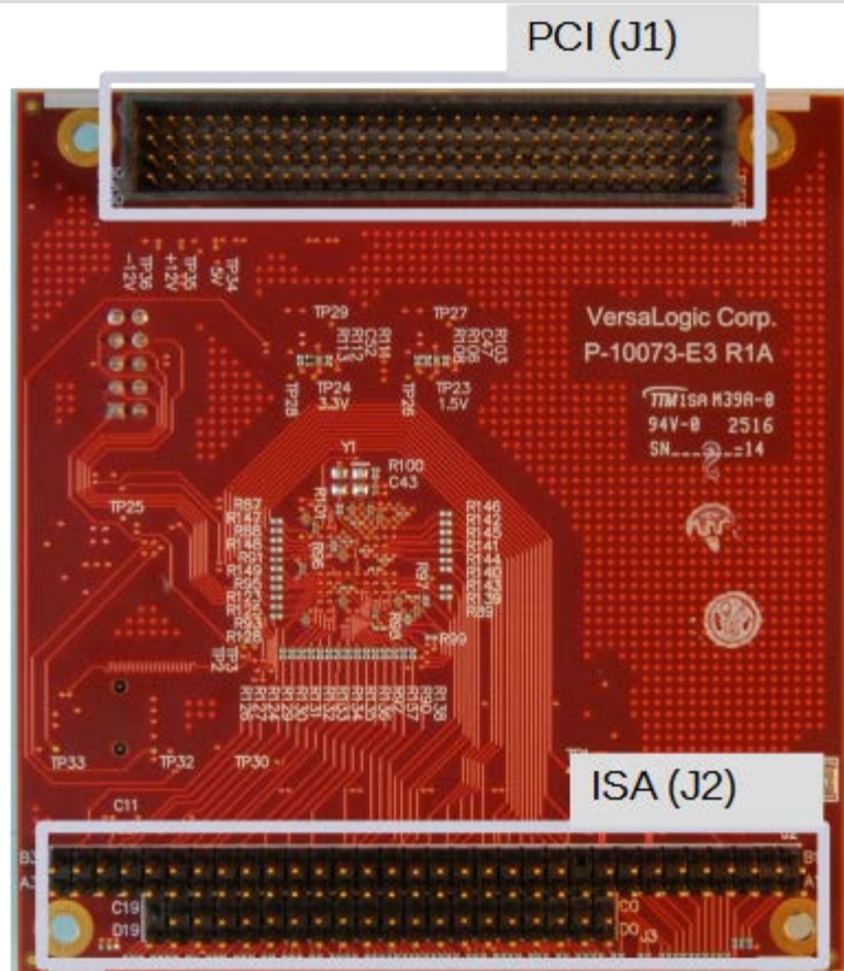
Figure 2. Major Components and Connectors (Bottom Side)
