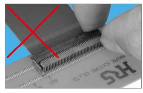
**5** Forces to the FPC after insertion and closing of the actuator.
