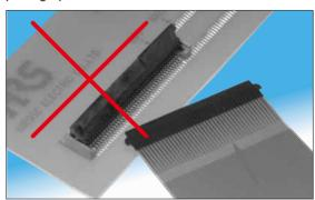
Properly insert the FPC positioning tabs into the corresponding areas on both sides of the insulator body.
