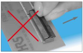
PFC Insertion and closing of the actuator.
