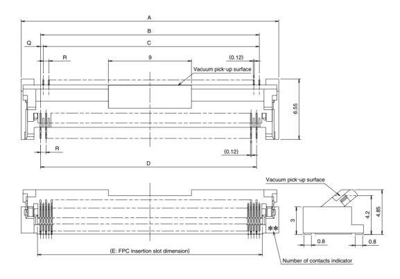
Notes 1: The coplanarity of each terminal lead is within 0.1.
