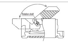
Be careful not to apply excessive force when operating the actuator from the open position (before the FPC has been inserted).
