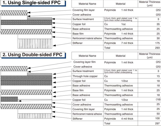
\* To prevent release of the FPC due to it's bending, use of the double-sided FPC with copper foil on the back side is NOT RECOMMENDED.
