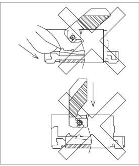
During the closing of the actuator do not pull up or push on it directly down.
