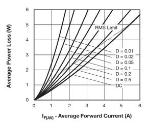
Fig. 5 - Forward Power Loss Characteristics
