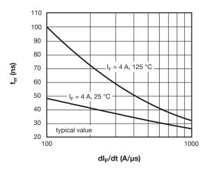
Fig. 6 - Typical Reverse Recovery vs. dI<sub>F</sub>/dt
