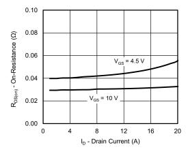
On-Resistance vs. Drain Current
