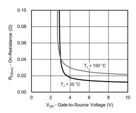
On-Resistance vs. Gate-to-Source Voltage
