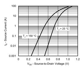
**Source Drain Diode Forward Voltage**
