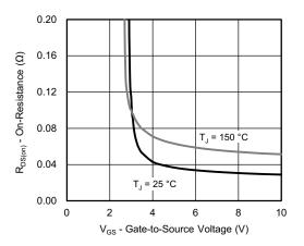
On-Resistance vs. Gate-to-Source Voltage
