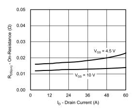
On-Resistance vs. Drain Current
