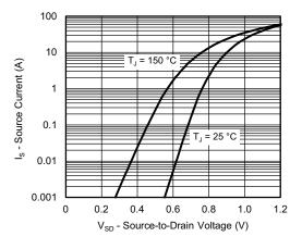
**Source Drain Diode Forward Voltage**
