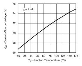
**Drain Source Breakdown vs. Junction Temperature**
