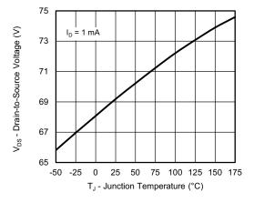
**Drain Source Breakdown vs. Junction Temperature**
