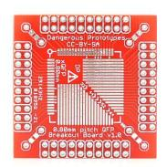
xQFP breakout board -0.8mm
