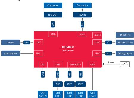
The block diagram shows the main components of the XMC4800 Automation Board V2 and their interconnections. The main building blocks are:
